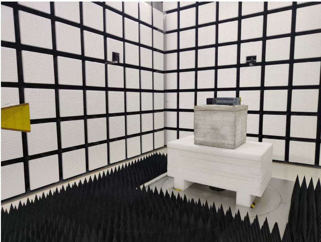
Radiated Emissions Above 1G rear View
