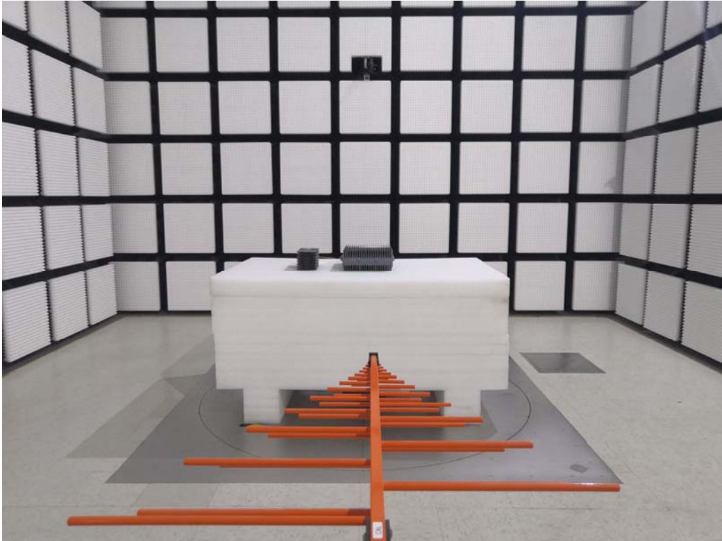
Radiated Emissions Above 1G rear View
