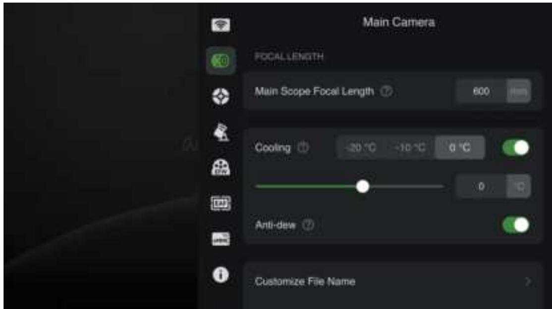
**Customize File Name:** You can customize the file name of the images you captured. The addible options include camera model, gain, temperature, etc.
