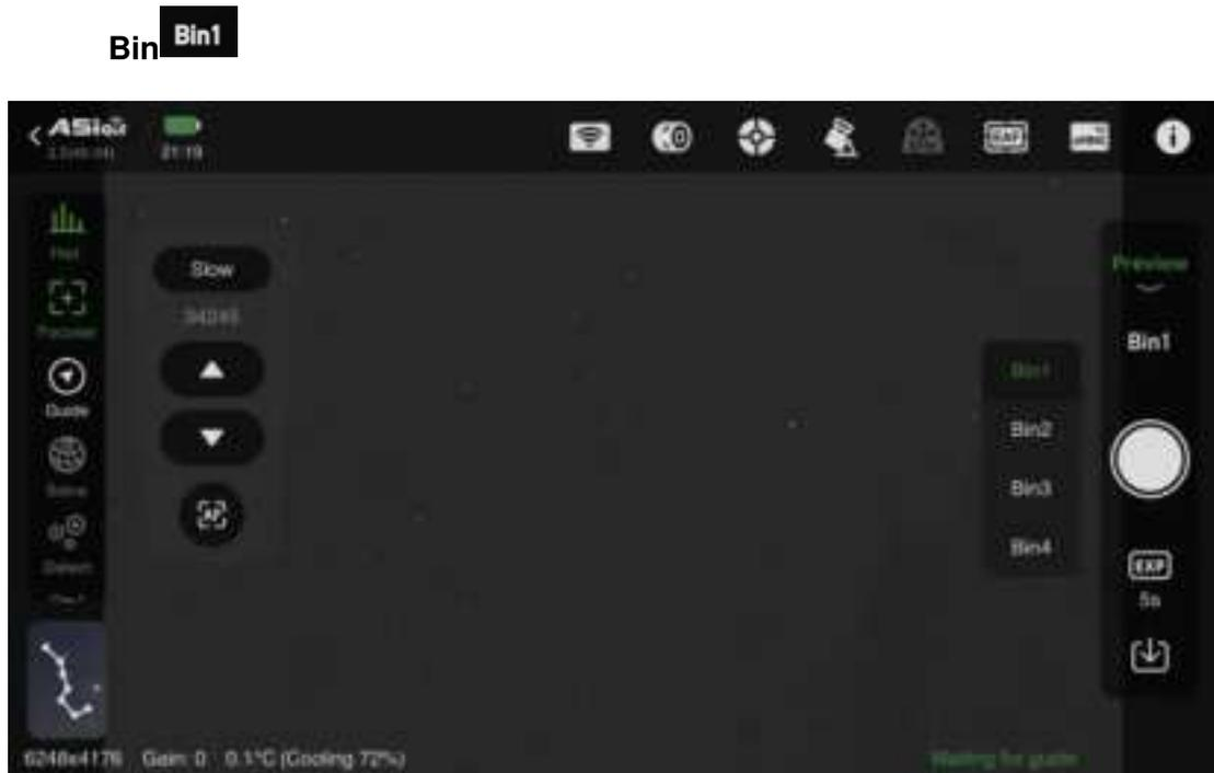
During fine focusing, adjust focus based on the principle that a smaller HFD value under Bin1 indicates better focus (can be adjusted from the MAX Bin down to Bin1).
