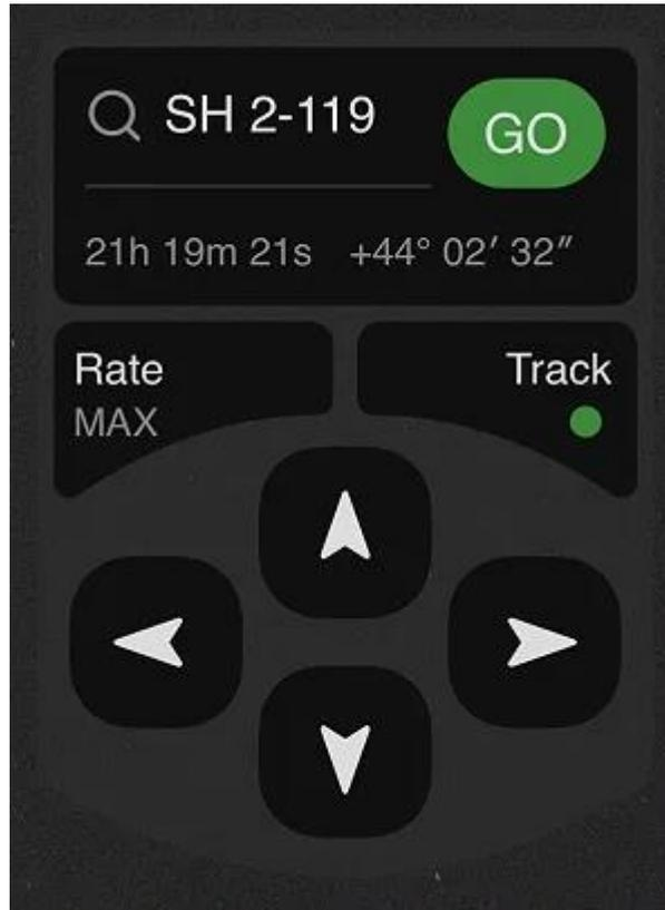
Direction Buttons and Speed Slider: These can be used together to select different movement speeds and move the mount's RA or DEC axis for preferred framing or other needs.
