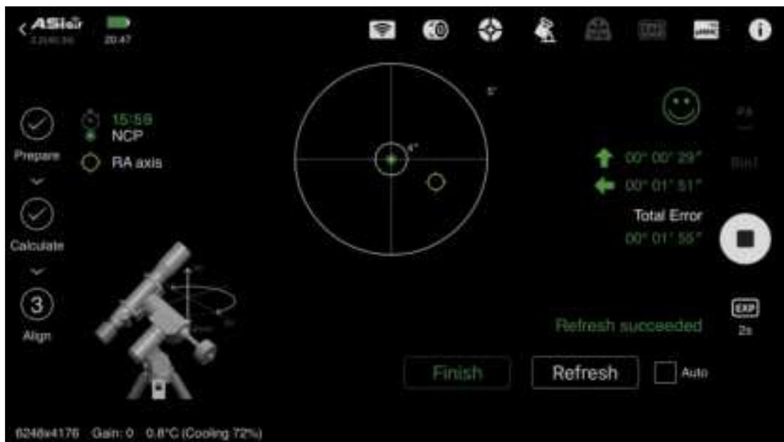
After the adjustment is completed, please tighten the azimuth lock screw and latitude adjustment knob in time. Tap Finish to obtain the ranking data.
