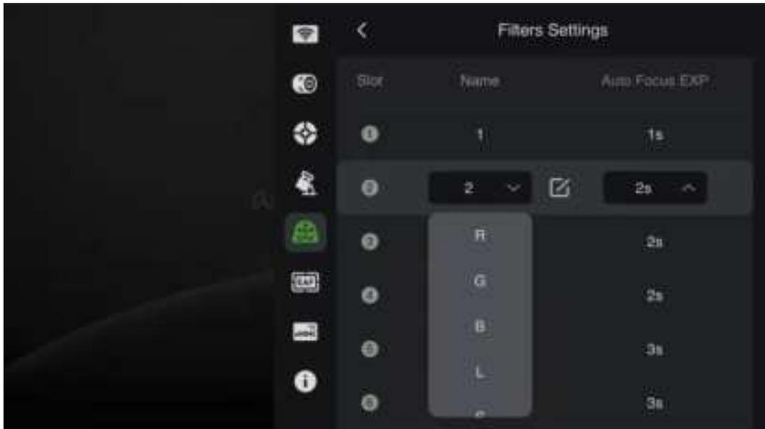
**Filters:** Set the name and autofocus exposure time for each filter position. You can choose names based on the filters you use or customize them.
