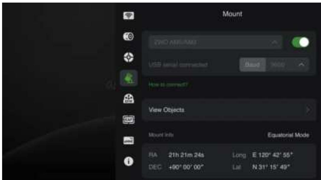
Select the corresponding mount model or connection method and toggle the switch to connect. For specific mount connection methods, refer to the "Connection Methods" section in this document.
