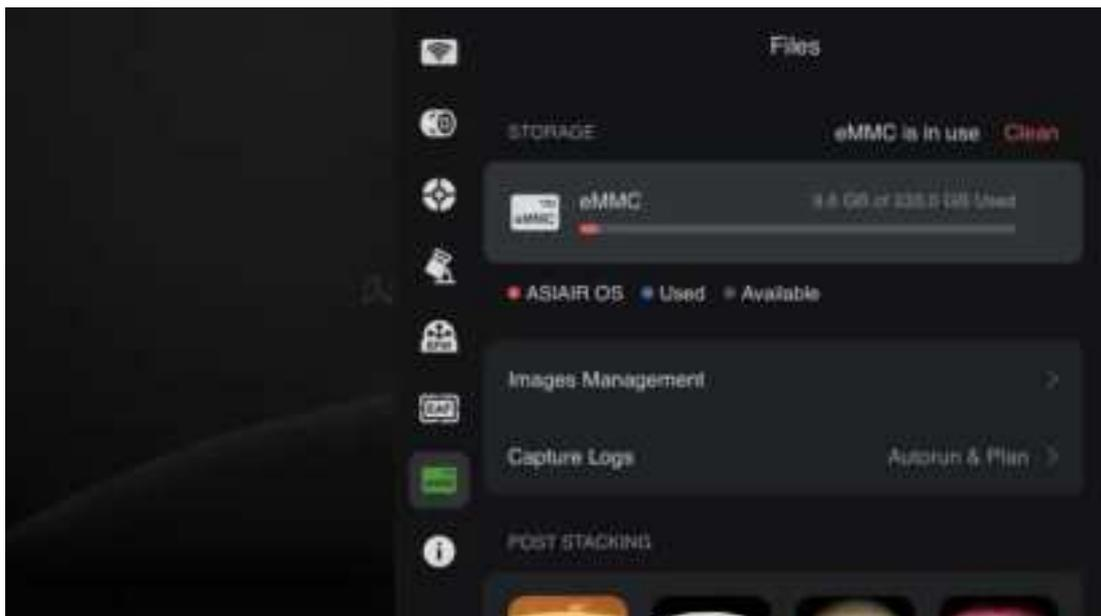
**Storage:** Displays the storage space and usage status of the wireless smart camera. The camera has built-in eMMC storage and also supports external USB storage devices.
