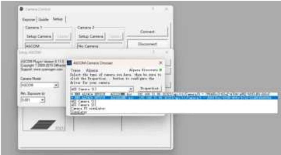
Click Connect to connect to the camera. Now you can control the camera on PC.
