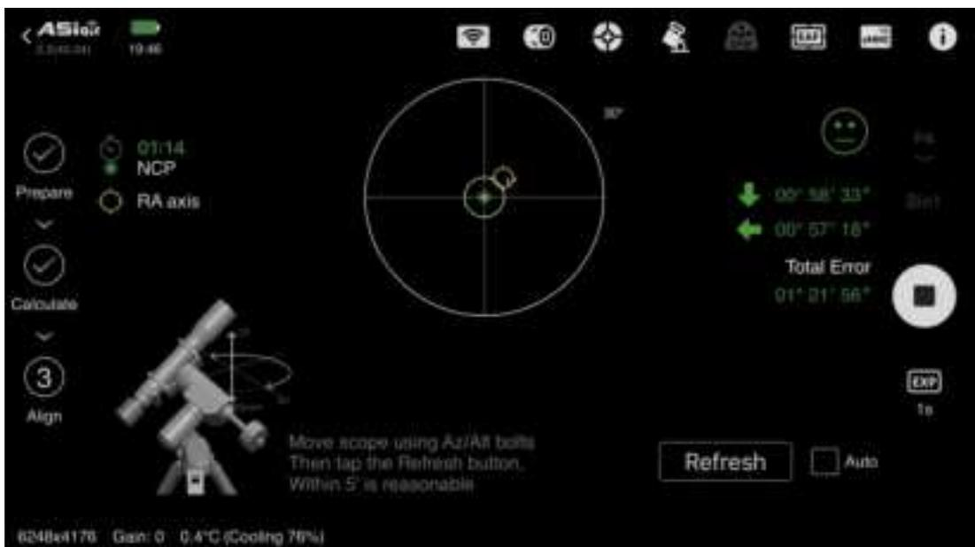
Adjust the mount according to the green numbers on the right side (loosen the mount's azimuth lock screws and latitude adjustment knobs
