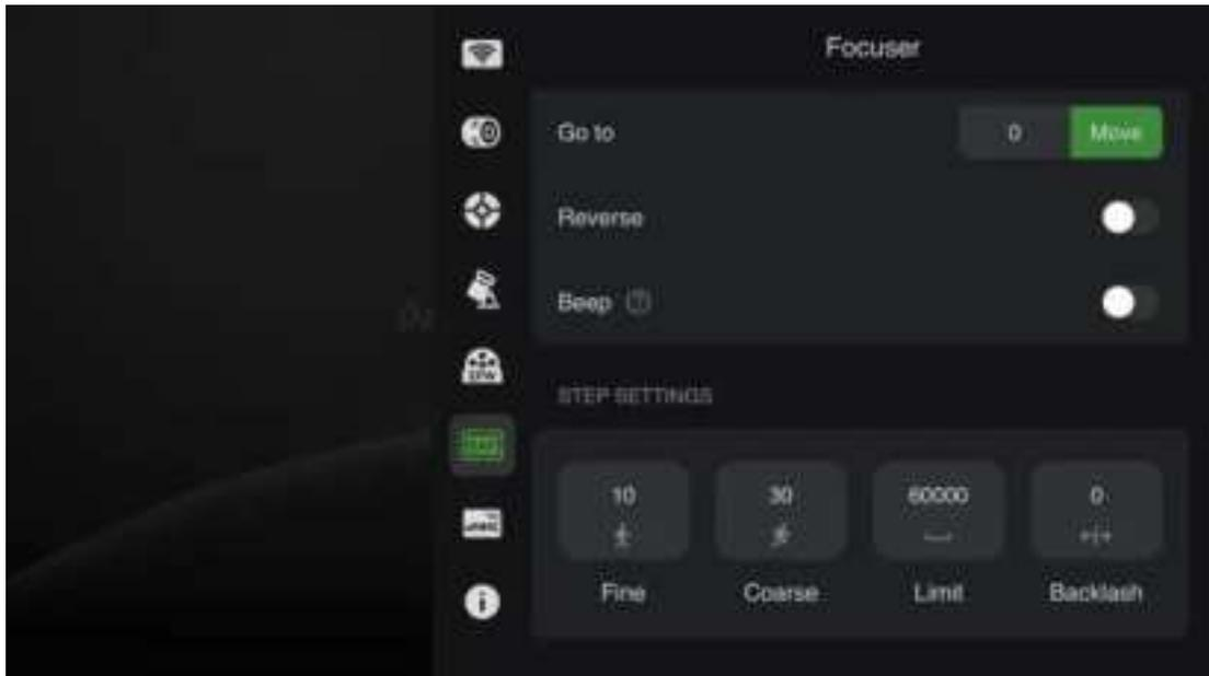
**Step Settings:** Configure the step count for fine-tuning and coarse adjustments. The travel limit refers to the maximum travel position that the EAF can move to.
