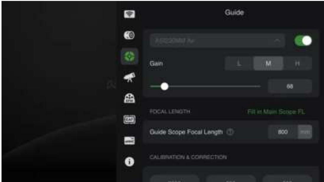
Select and turn on the guide camera here. It is recommended to select "High" for gain. In wireless smart camera products, please be sure to fill in the focal length of the guide camera accurately.
