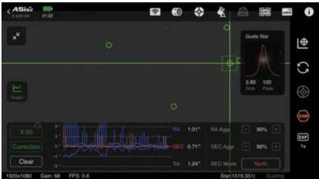
We can tap
