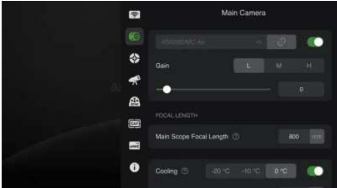
Select the main camera and turn it on. When switching cameras, please turn the switch off first, then turn it on after switching cameras.
