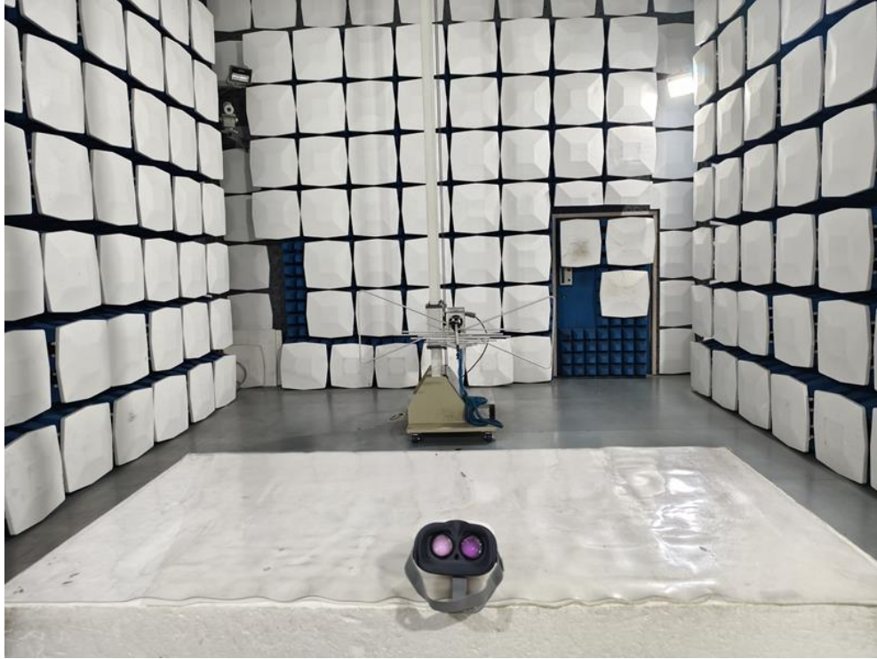
Radiated Emission Test Setup:
