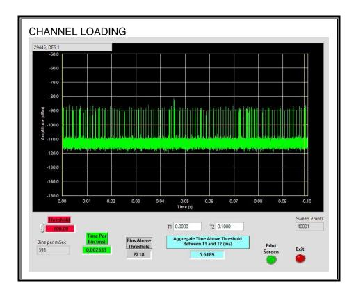
The level of traffic loading on the channel by the EUT is 5.618%
