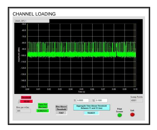
The level of traffic loading on the channel by the EUT is 18.66%
