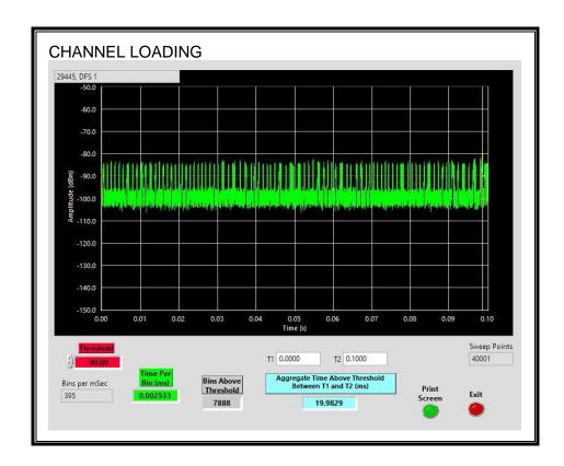
The level of traffic loading on the channel by the EUT is 19.98%
