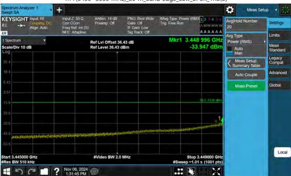
n77(3450~3550 MHz)\_20 M\_Band Edge\_Low\_BPSK\_1RB(2)
