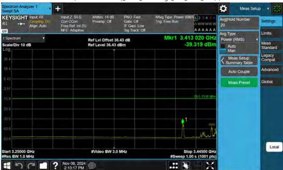
n77(3450~3550 MHz)\_40 M\_Band Edge\_Low\_BPSK\_1RB(3)
