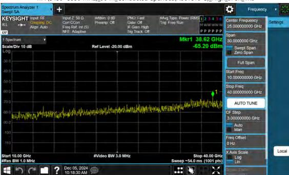
n77(3450~3550 MHz)\_90 M\_Conducted Spurious(Above10 G)\_High\_BPSK\_1RB
