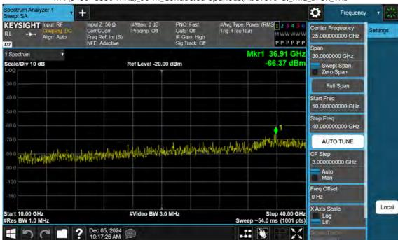
n77(3450~3550 MHz)\_90 M\_Conducted Spurious(Above10 G)\_Mid\_BPSK\_1RB
