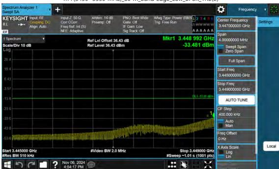
n77(3450~3550 MHz)\_80 M\_Band Edge\_Low\_BPSK\_1RB(2)
