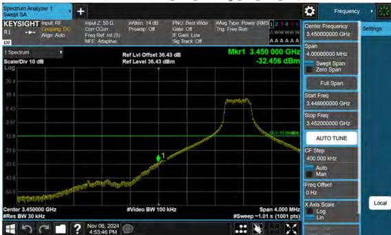
n77(3450~3550 MHz)\_80 M\_Band Edge\_Low\_BPSK\_1RB(1)
