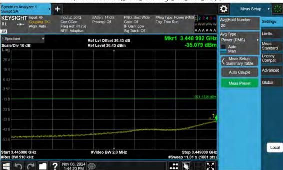
n77(3450~3550 MHz)\_30 M\_Band Edge\_Low\_BPSK\_1RB(2)
