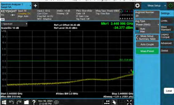
n77(3450~3550 MHz)\_40 M\_Band Edge\_Low\_BPSK\_1RB(2)
