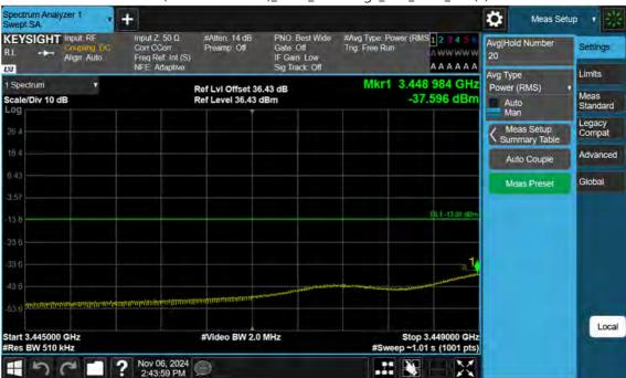
n77(3450~3550 MHz)\_50 M\_Band Edge\_Low\_BPSK\_1RB(2)
