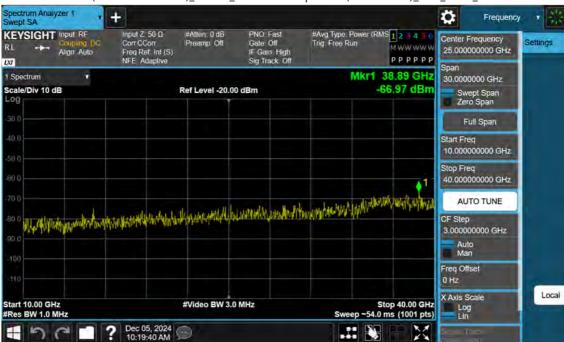
n77(3450~3550 MHz)\_100 M\_Conducted Spurious(Above10 G)\_Low\_BPSK\_1RB
