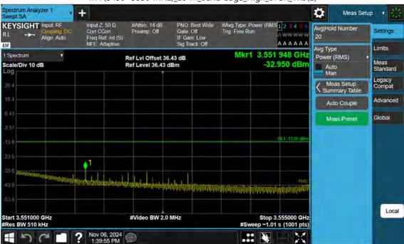
n77(3450~3550 MHz)\_20 M\_Band Edge\_High\_BPSK\_1RB(2)
