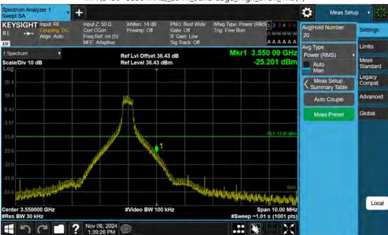
n77(3450~3550 MHz)\_20 M\_Band Edge\_High\_BPSK\_1RB(1)
