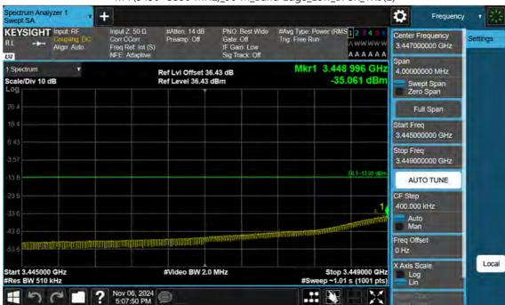
n77(3450~3550 MHz)\_90 M\_Band Edge\_Low\_BPSK\_1RB(2)
