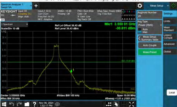
n77(3450~3550 MHz)\_30 M\_Band Edge\_High\_BPSK\_1RB(1)
