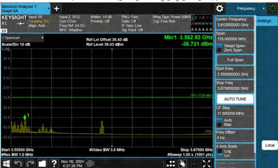
n77(3450~3550 MHz)\_60 M\_Band Edge\_High\_BPSK\_1RB(3)
