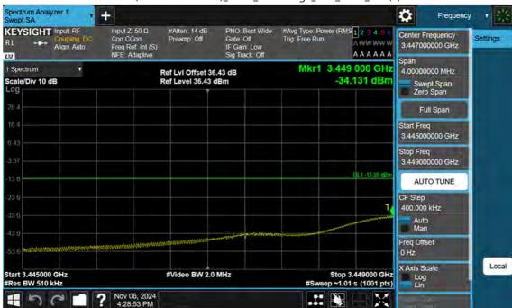
n77(3450~3550 MHz)\_60 M\_Band Edge\_Low\_BPSK\_1RB(2)
