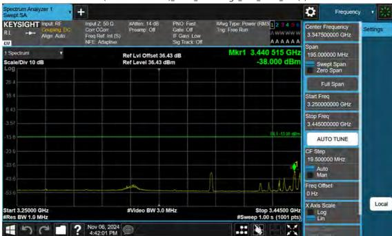
n77(3450~3550 MHz)\_70 M\_Band Edge\_Low\_BPSK\_1RB(3)
