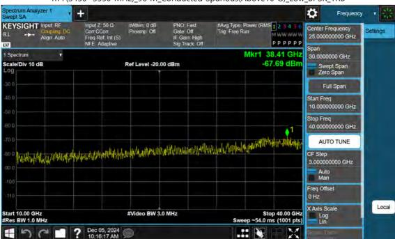
n77(3450~3550 MHz)\_90 M\_Conducted Spurious(Above10 G)\_Low\_BPSK\_1RB
