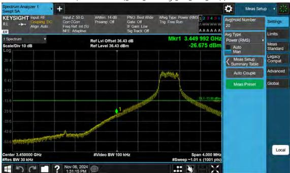
n77(3450~3550 MHz)\_20 M\_Band Edge\_Low\_BPSK\_1RB(1)
