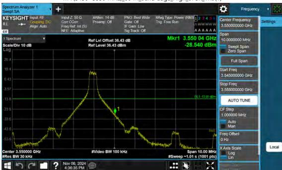
n77(3450~3550 MHz)\_60 M\_Band Edge\_High\_BPSK\_1RB(1)
