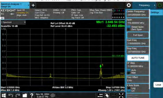
n77(3450~3550 MHz)\_100 M\_Band Edge\_High\_BPSK\_1RB(3)
