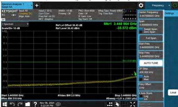
n77(3450~3550 MHz)\_100 M\_Band Edge\_Low\_BPSK\_1RB(2)
