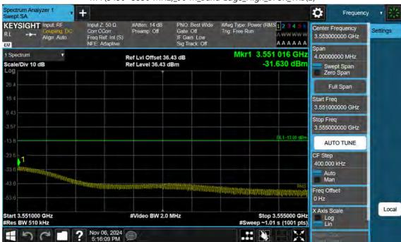
n77(3450~3550 MHz)\_90 M\_Band Edge\_High\_BPSK\_1RB(2)
