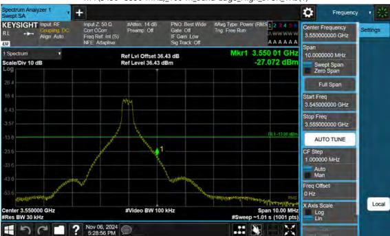
n77(3450~3550 MHz)\_100 M\_Band Edge\_High\_BPSK\_1RB(1)
