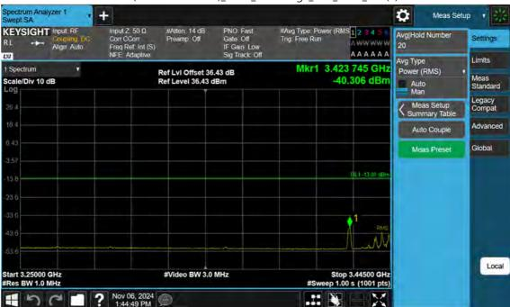
n77(3450~3550 MHz)\_30 M\_Band Edge\_Low\_BPSK\_1RB(3)
