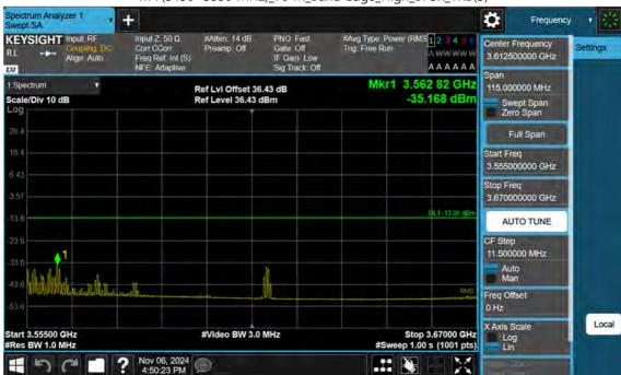
n77(3450~3550 MHz)\_70 M\_Band Edge\_High\_BPSK\_1RB(3)
