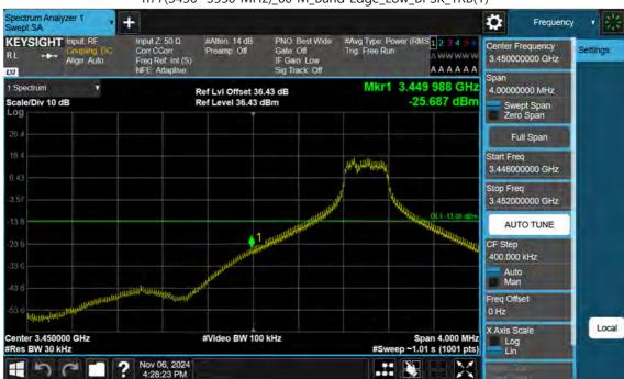
n77(3450~3550 MHz)\_60 M\_Band Edge\_Low\_BPSK\_1RB(1)
