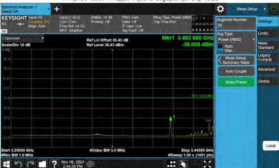
n77(3450~3550 MHz)\_50 M\_Band Edge\_Low\_BPSK\_1RB(3)
