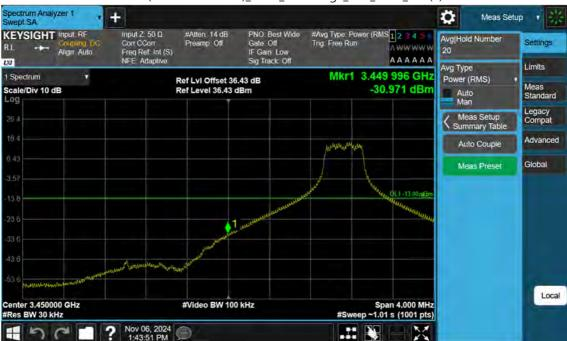
n77(3450~3550 MHz)\_30 M\_Band Edge\_Low\_BPSK\_1RB(1)
