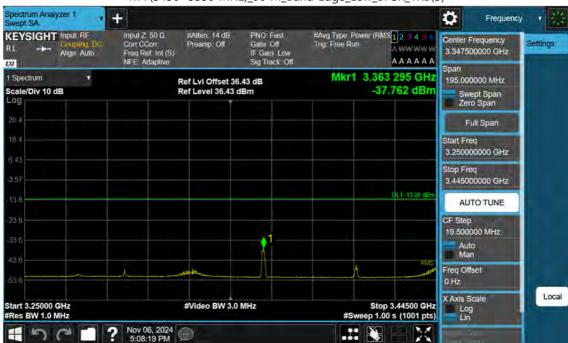
n77(3450~3550 MHz)\_90 M\_Band Edge\_Low\_BPSK\_1RB(3)
