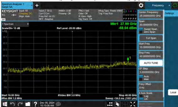
n77(3450~3550 MHz)\_80 M\_Conducted Spurious(Above10 G)\_High\_BPSK\_1RB
