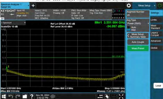
n77(3450~3550 MHz)\_50 M\_Band Edge\_High\_BPSK\_1RB(2)
