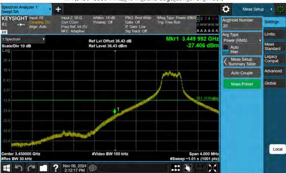
n77(3450~3550 MHz)\_40 M\_Band Edge\_Low\_BPSK\_1RB(1)
