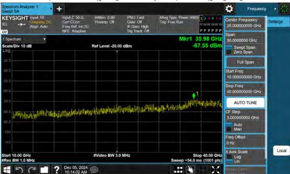
n77(3450~3550 MHz)\_80 M\_Conducted Spurious(Above10 G)\_Mid\_BPSK\_1RB
