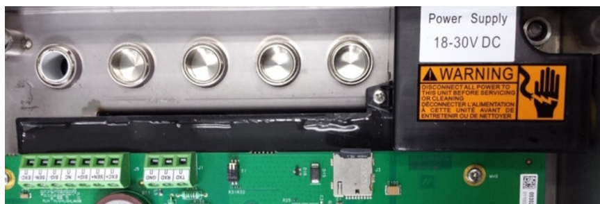
Figure 2-5: DC Power input Connector with Cover
