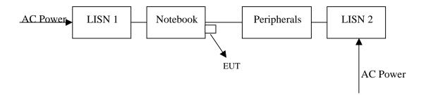
The EUT are connected to the main power through a line impedance stabilization network (LISN). This provides a 50 ohm/50uH coupling impedance for the measuring equipment. The peripheral devices are also connected to the main power through a LISN that provides a 50ohm/50uH coupling impedance with 50ohm termination. Both sides (Line and Neutral) of AC line are checked for maximum conducted interference. In order to find the maximum emission, the relative positions of
