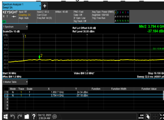
N2(5M)_DFT-s- OFDM BPSK Edge 1RB Left Low CH
