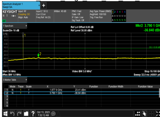
N2(5M)_DFT-s- OFDM BPSK Edge 1RB Left Mid CH
