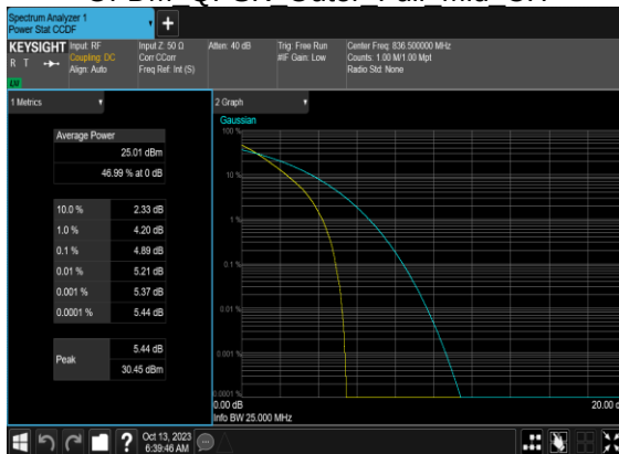
N5(20M)_DFT-s-OFDM QPSK Outer Full Mid CH
