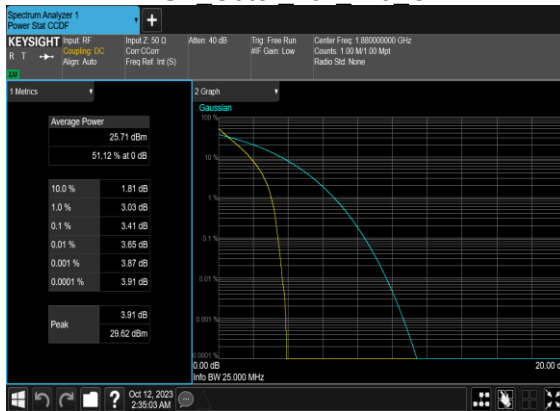
N2(20M)_DFT-s-OFDM_PI_2-BPSK Outer Full Mid CH
