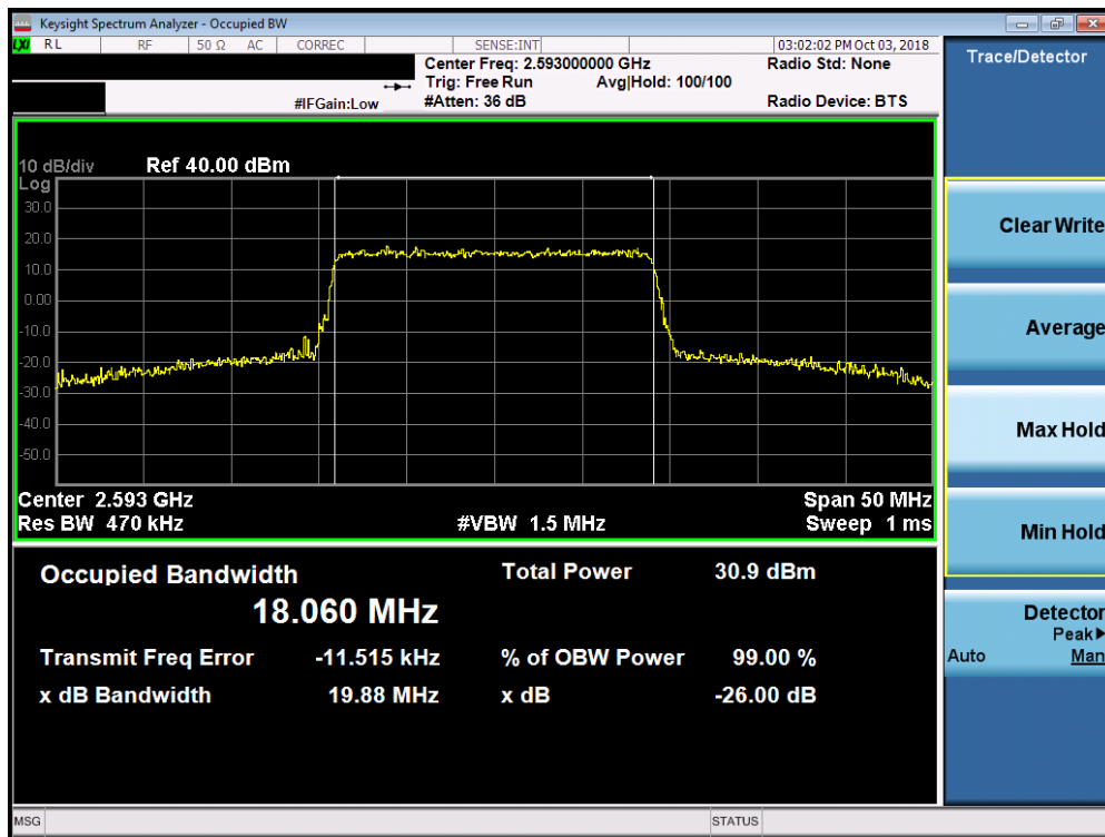
Plot 7-61. Occupied Bandwidth Plot (Band 41 - 20.0MHz 16-QAM - Full RB Configuration)
