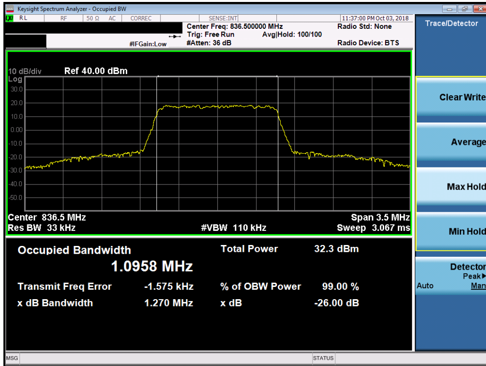
Plot 7-12. Occupied Bandwidth Plot (Band 26/5 - 1.4MHz QPSK - Full RB Configuration)
