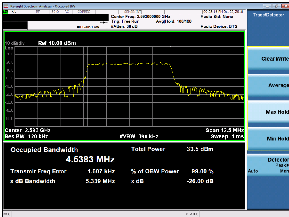
Plot 7-47. Occupied Bandwidth Plot (Band 41 - 5.0MHz 16-QAM - Full RB Configuration)
