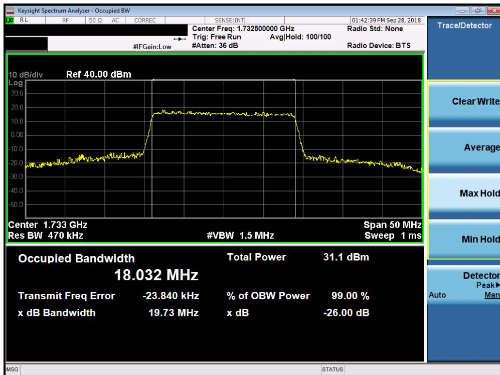
Plot 7-33. Occupied Bandwidth Plot (Band 4 - 20.0MHz 16-QAM - Full RB Configuration)
