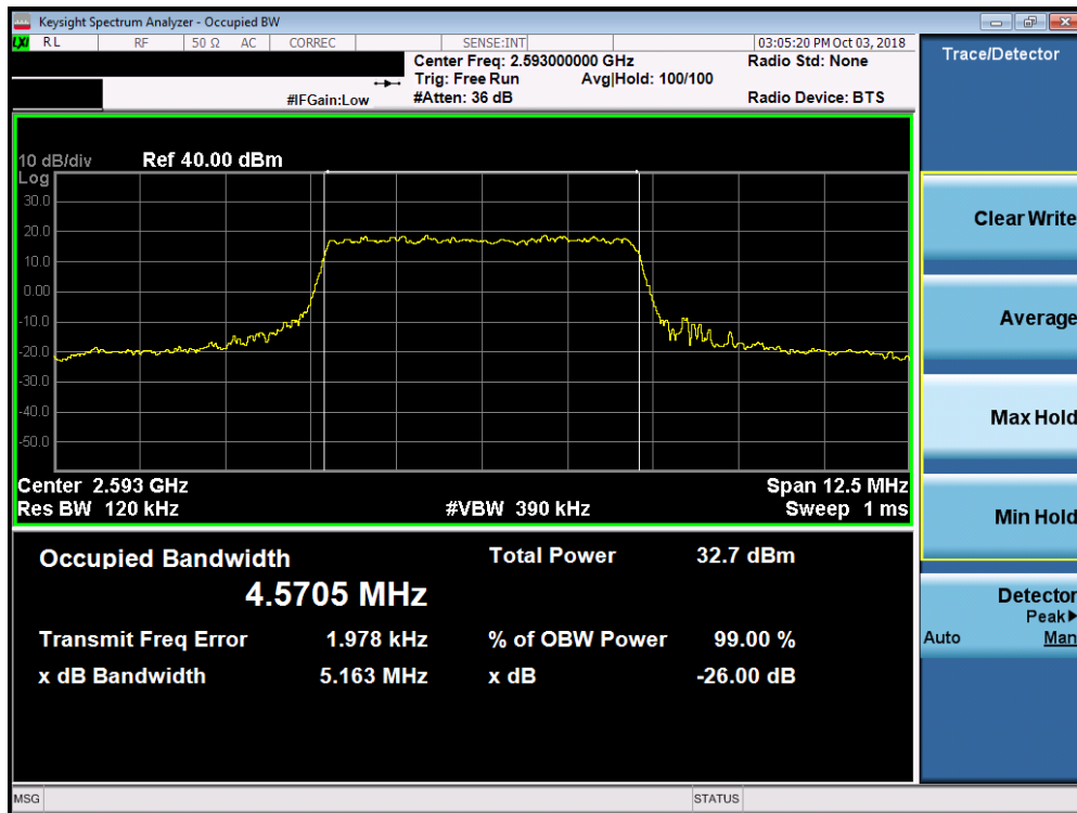
Plot 7-54. Occupied Bandwidth Plot (Band 41 - 5.0MHz QPSK - Full RB Configuration)
