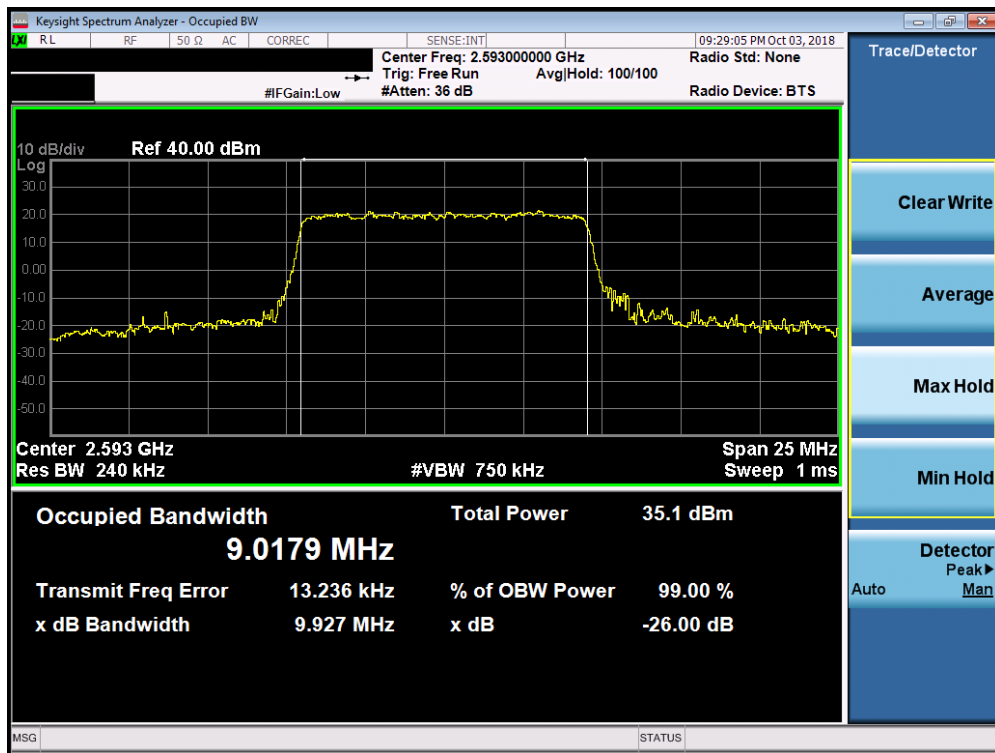
Plot 7-48. Occupied Bandwidth Plot (Band 41 - 10.0MHz QPSK - Full RB Configuration)
