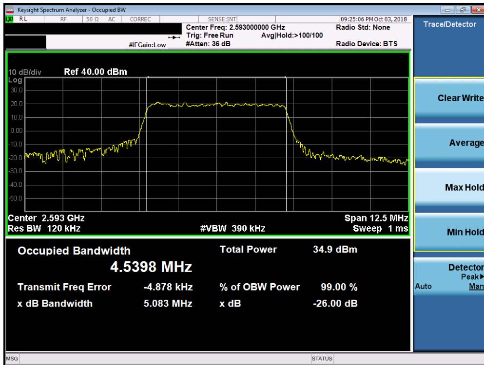
Plot 7-46. Occupied Bandwidth Plot (Band 41 - 5.0MHz QPSK - Full RB Configuration)
