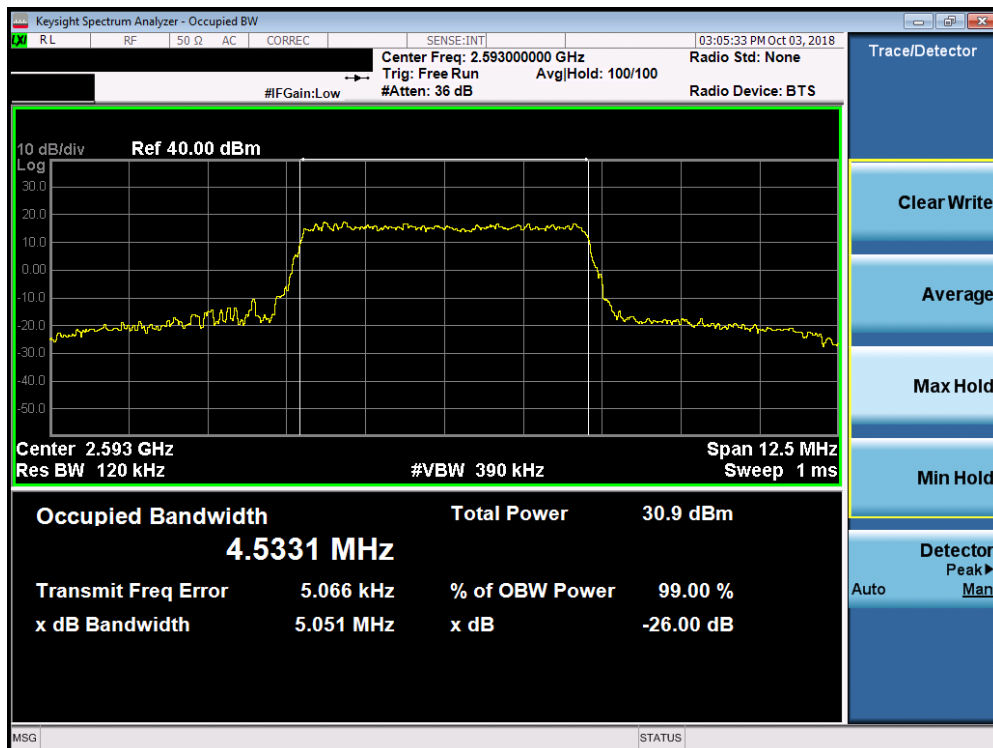
Plot 7-55. Occupied Bandwidth Plot (Band 41 - 5.0MHz 16-QAM - Full RB Configuration)
