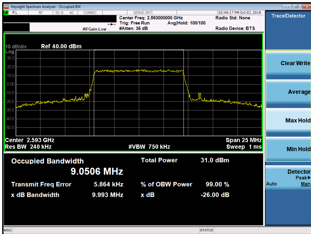
Plot 7-57. Occupied Bandwidth Plot (Band 41 - 10.0MHz 16-QAM - Full RB Configuration)
