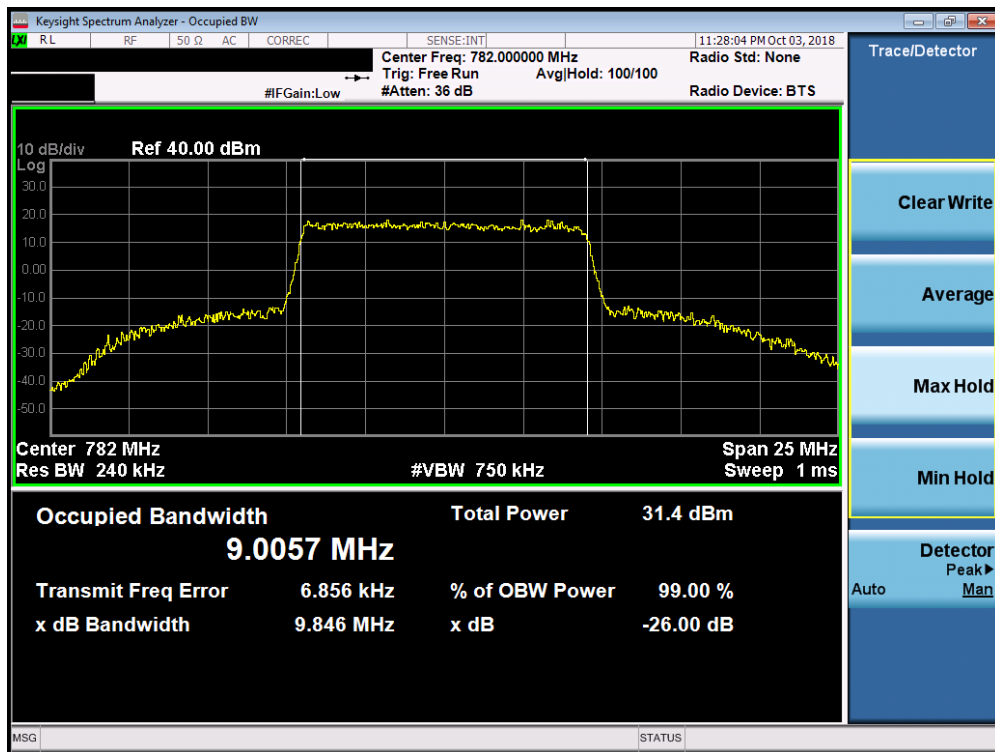
Plot 7-11. Occupied Bandwidth Plot (Band 13 - 10.0MHz 16-QAM - Full RB Configuration)
