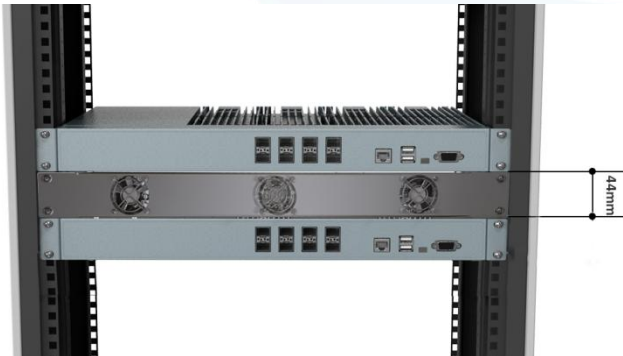
Figure 6. Separation of adjacent A2s
