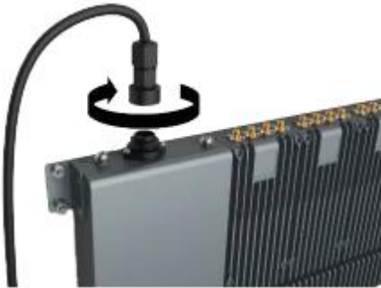
Figure 12. Connect power cable at rear side
