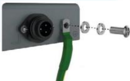
Figure 8. Connect Ground Cable at Rear Side
