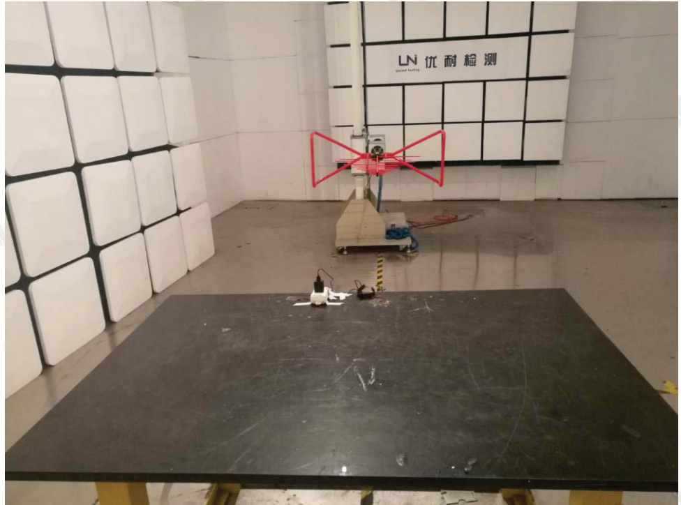
Radiated Emission (Below 1G)
