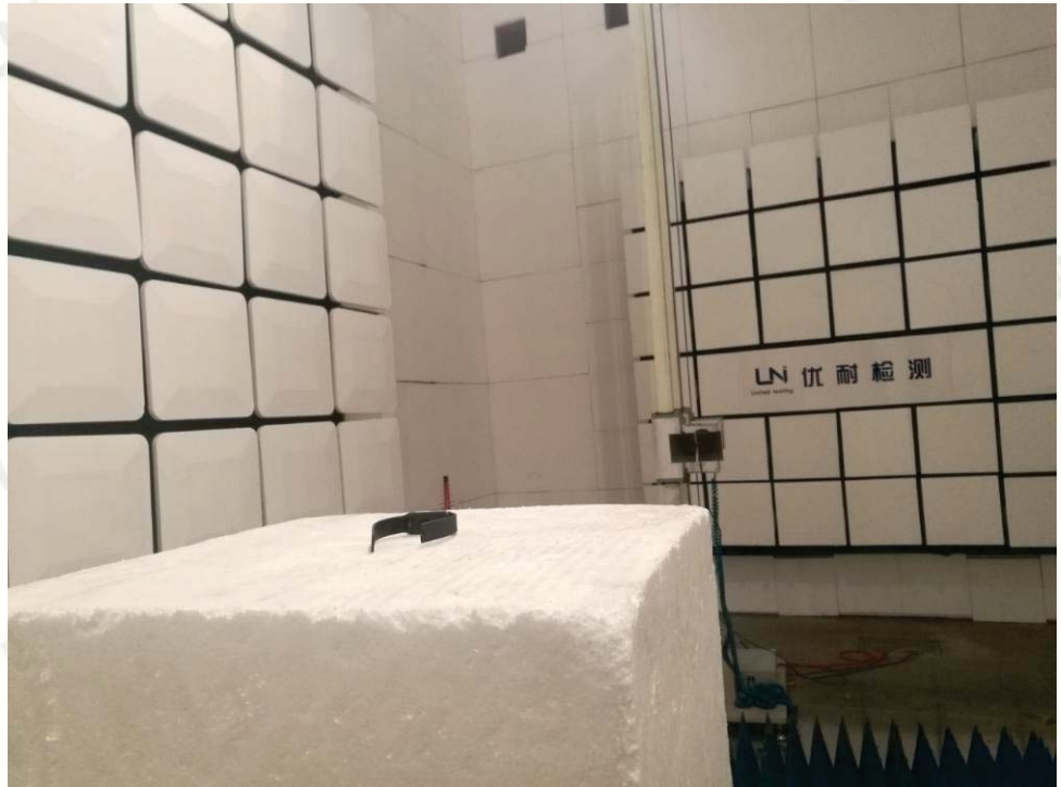
Radiated Emission (Above 1G)
