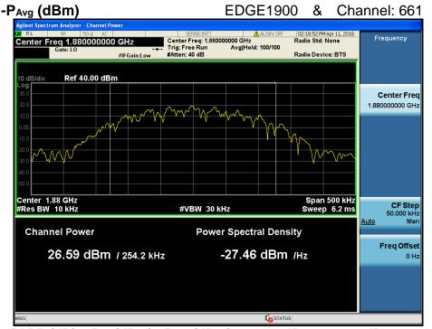
$PAPR(dB) = P_{Pk}(dBm) - P_{Avg}(dBm) = 30.05 dBm - 26.59 dBm = 3.40 dB$
