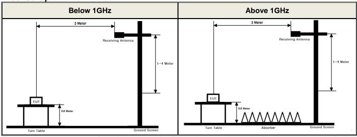
These measurements were performed at 3 m test site. The equipment under test is placed on a non-conductive table 0.8 meters above a turntable which is flush with the ground plane and 3 meters from the receive antenna. For measurements above 1GHz absorbers are placed on the floor between the turn table and the antenna mast in such a way so as to maximize the reduction of reflections. For measurements below 1 GHz, the absorbers are removed.
