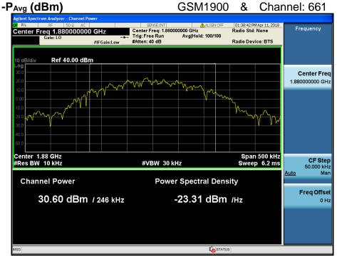
$PAPR (dB) = P_{Pk} (dBm) - P_{Avg} (dBm) = 30.84 dBm - 30.60 dBm = 0.24 dB$
