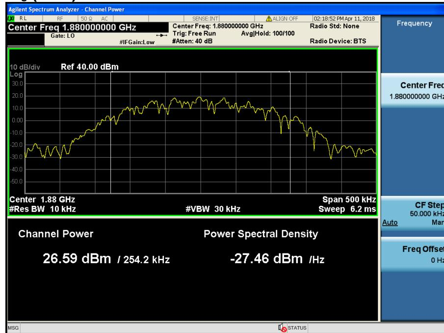
$$PAPR (dB) = P_{Pk} (dBm) - P_{Avg} (dBm) = 30.05 \text{ dBm} - 26.59 \text{ dBm} = 3.40 \text{ dB}$$
