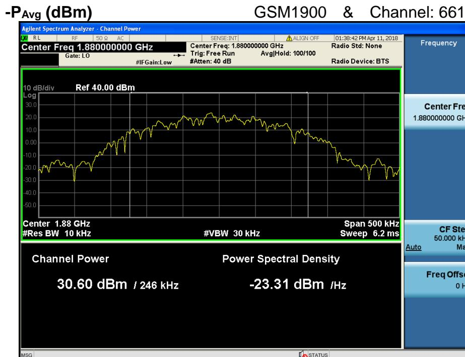
$$\text{PAPR (dB)} = \text{P}_{\text{Pk}} (\text{dBm}) - \text{P}_{\text{Avg}} (\text{dBm}) = 30.84 \text{ dBm} - 30.60 \text{ dBm} = 0.24 \text{ dB}$$
