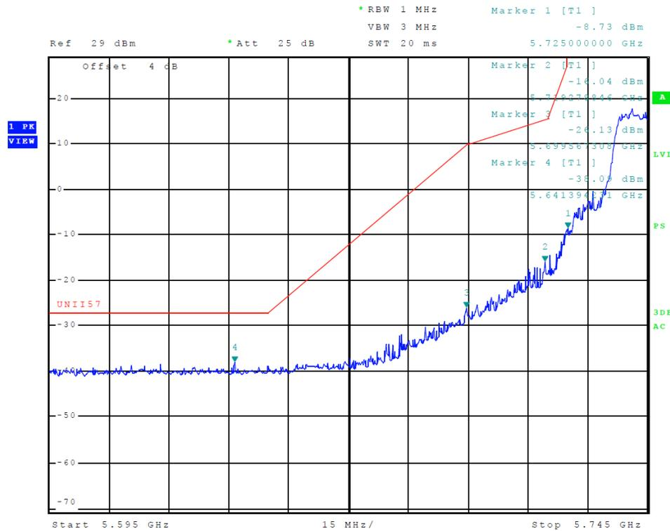
**Figure 28 Plot of Transmitter Low Band Edge (5725-5850 MHz Band, Chain 1, 802.11a)**
