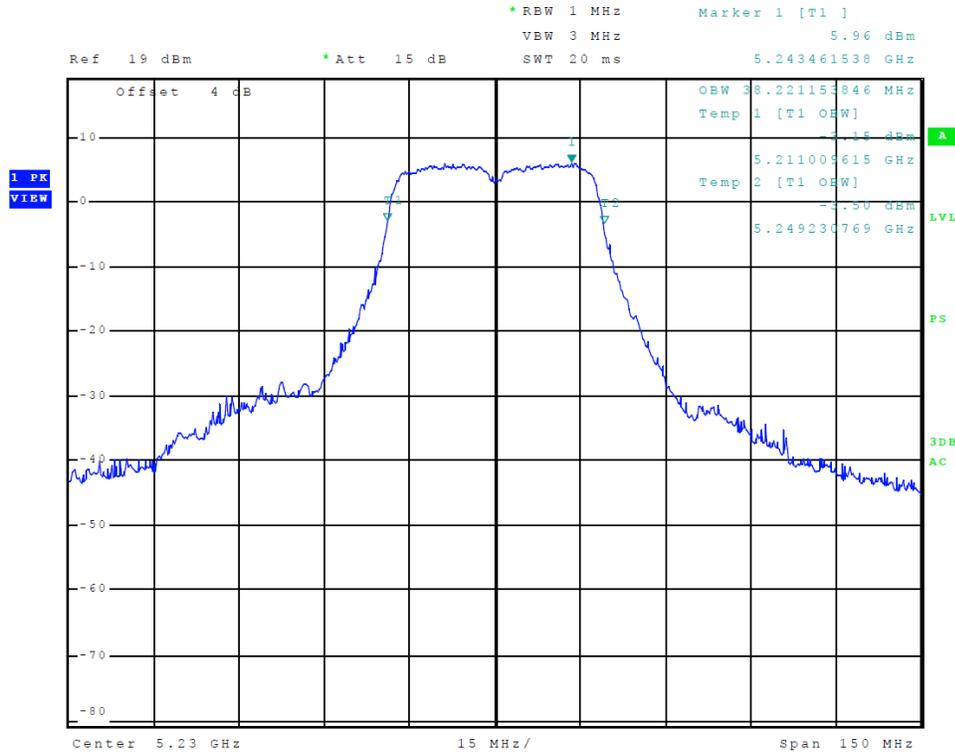
**Figure 19 Plot of Transmitter Emissions (5150-5250 MHz Band, 802.11n40, Chain 0, 99% OBW)**
