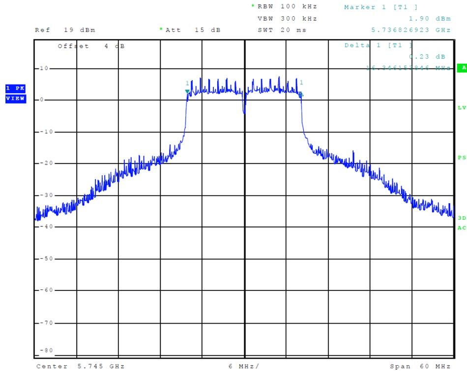
**Figure 38 Plot of Transmitter Emissions (5725-5850 MHz Band, 802.11a, Chain 1, 6-dB OBW)**
