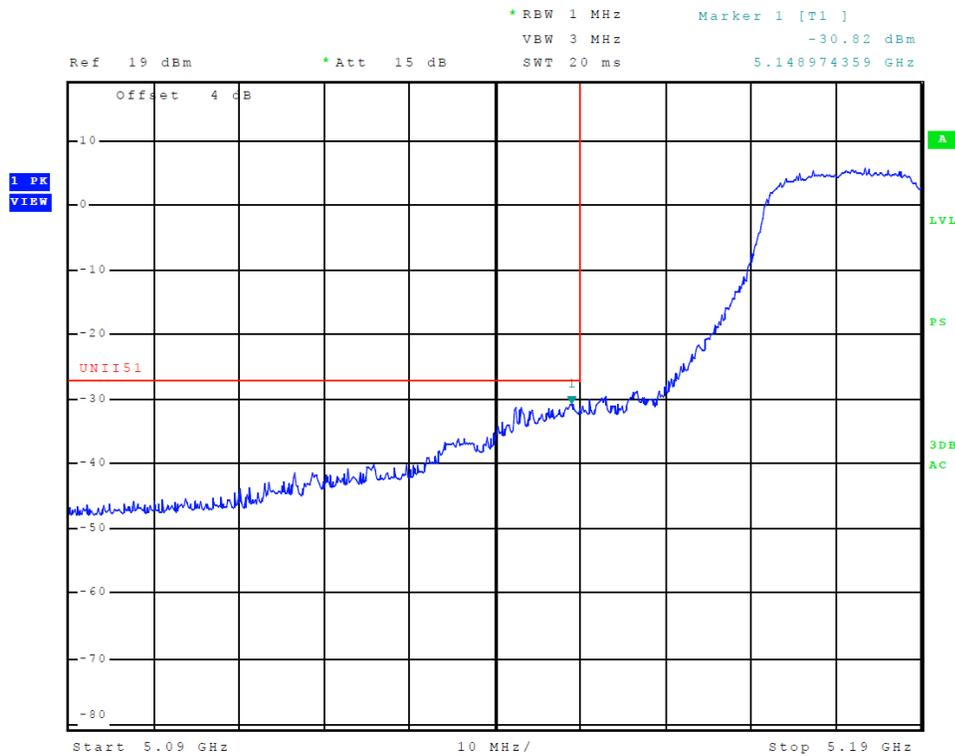
**Figure 9 Plot of Transmitter Low Band Edge (5150-5250 MHz Band, Chain 0, 802.11n40)**
