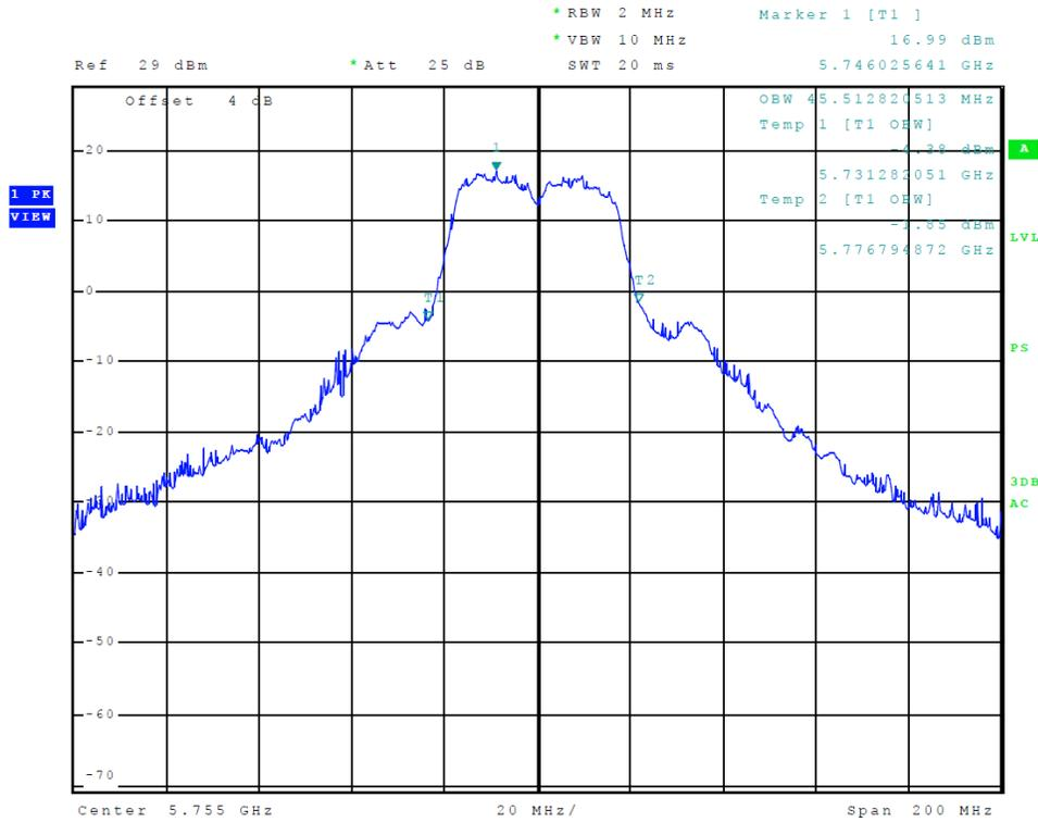
**Figure 39 Plot of Transmitter Emissions (5725-5850 MHz Band, 802.11n40, Chain 0, 99% OBW)**
