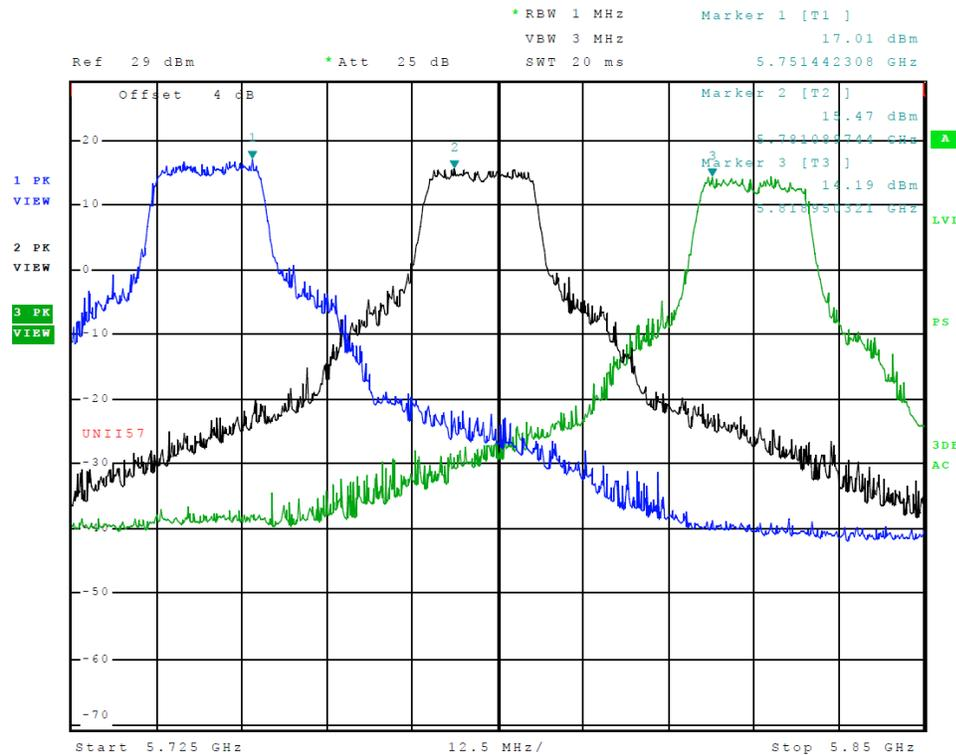
Figure 24 Plot of Transmitter Emissions (Across 5725-5850 MHz Band, Chain 1, 802.11a)
