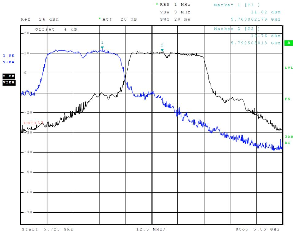
**Figure 25 Plot of Transmitter Emissions (Across 5725-5850 MHz Band, Chain 0, 802.11n40)**
