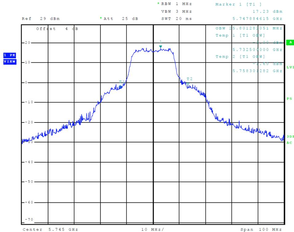
Figure 36 Plot of Transmitter Emissions (5725-5850 MHz Band, 802.11a, Chain 1, 99% OBW)
