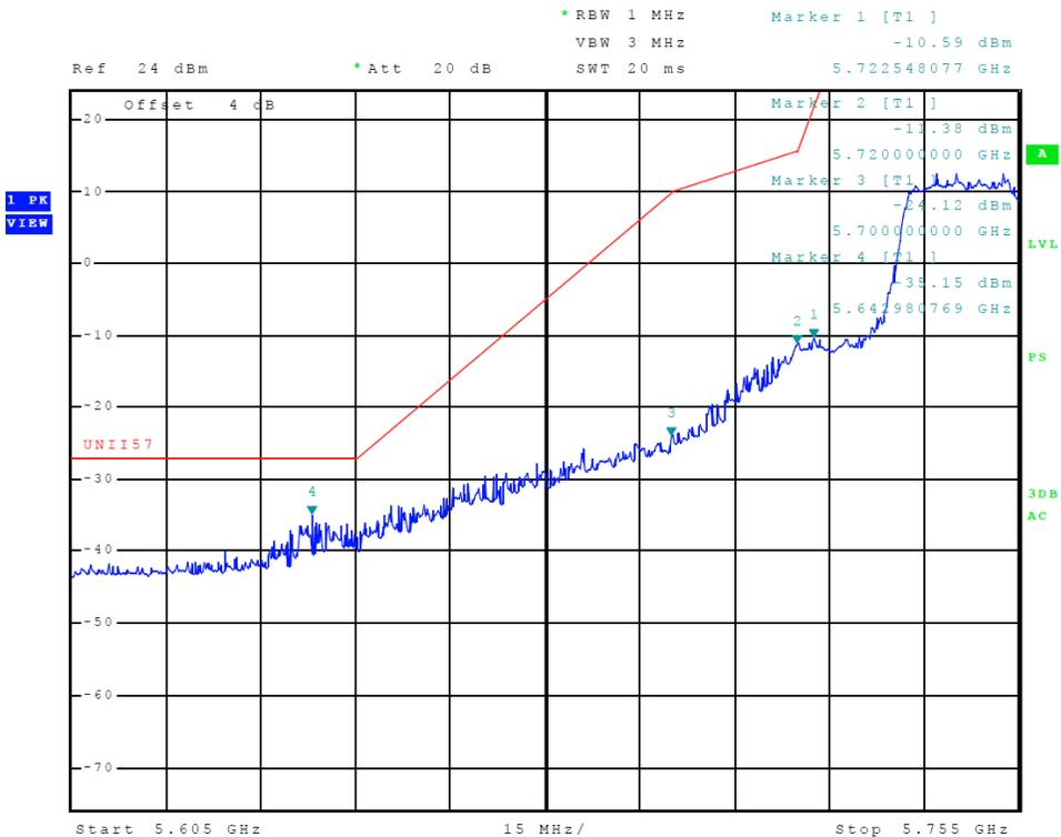
**Figure 30 Plot of Transmitter Low Band Edge (5725-5850 MHz Band, Chain 1, 802.11n40)**
