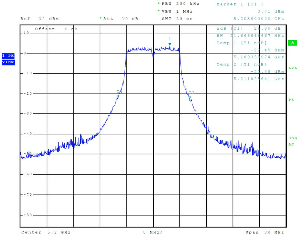
Figure 18 Plot of Transmitter Emissions (5150-5250 MHz Band, 802.11a, Chain 1, 26 dB OBW)
