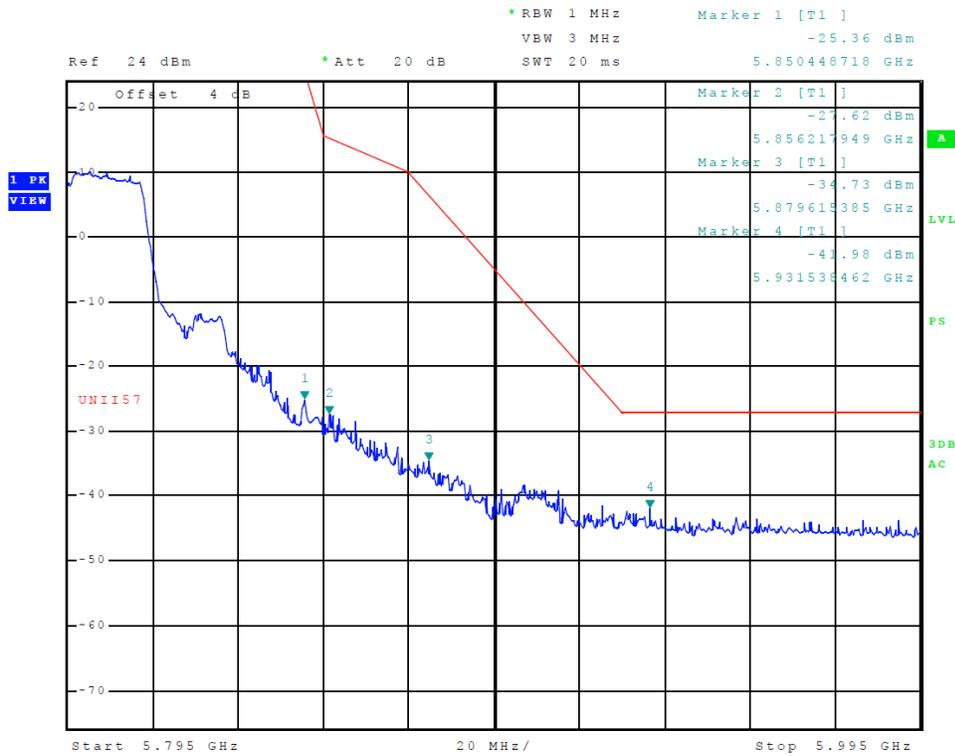
**Figure 33 Plot of Transmitter High Band Edge (5725-5850 MHz Band, Chain 0, 802.11n40)**
