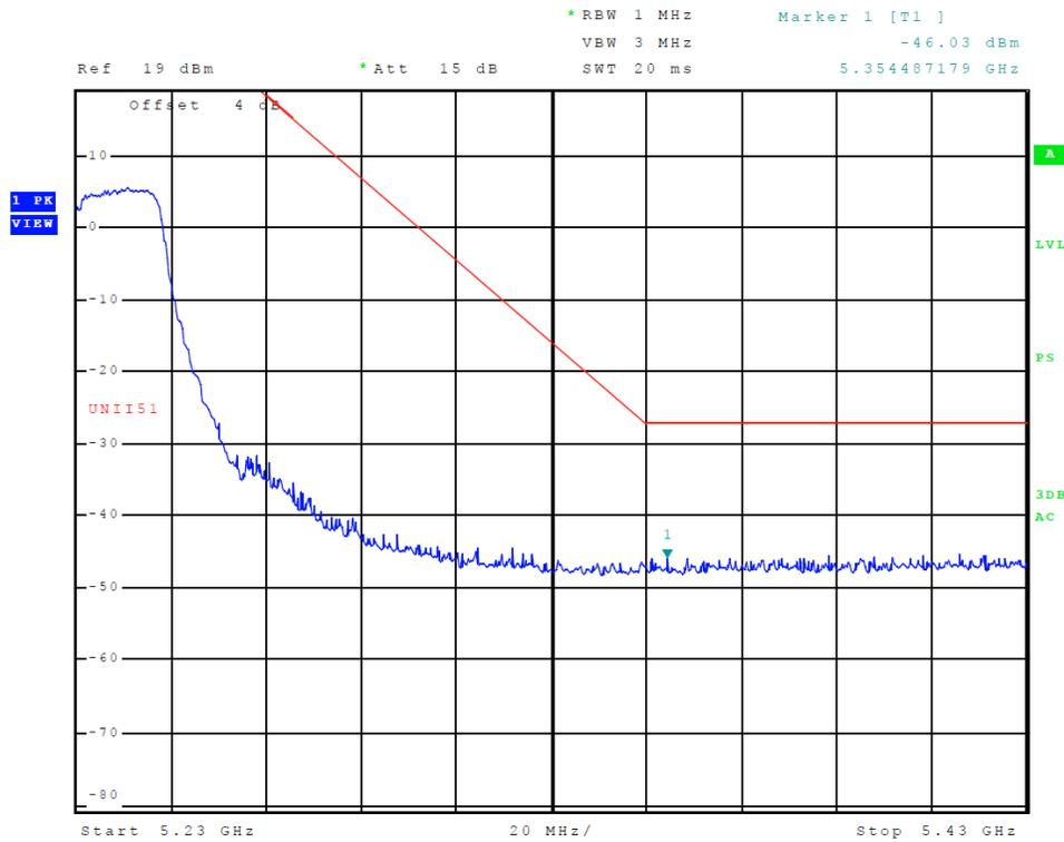
**Figure 13 Plot of Transmitter High Band Edge (5150-5250 MHz Band, Chain 0, 802.11n40)**
