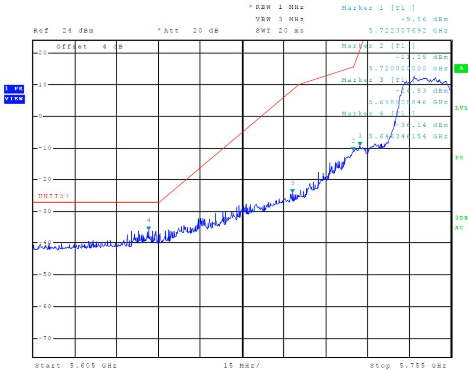
**Figure 29 Plot of Transmitter Low Band Edge (5725-5850 MHz Band, Chain 0, 802.11n40)**
