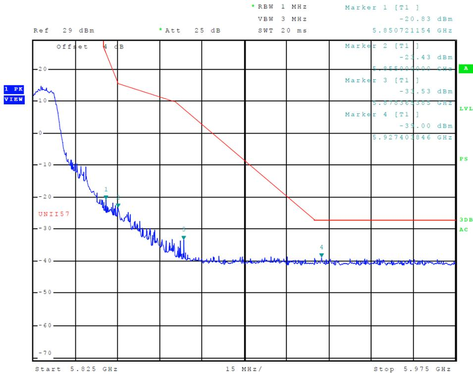
Figure 31 Plot of Transmitter High Band Edge (5725-5850 MHz Band, Chain 0, 802.11a)
