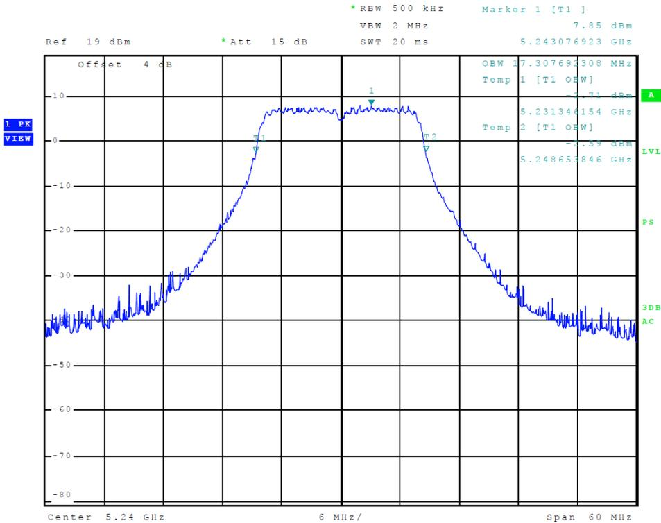
**Figure 16 Plot of Transmitter Emissions (5150-5250 MHz Band, 802.11a, Chain 1, 99% OBW)**
