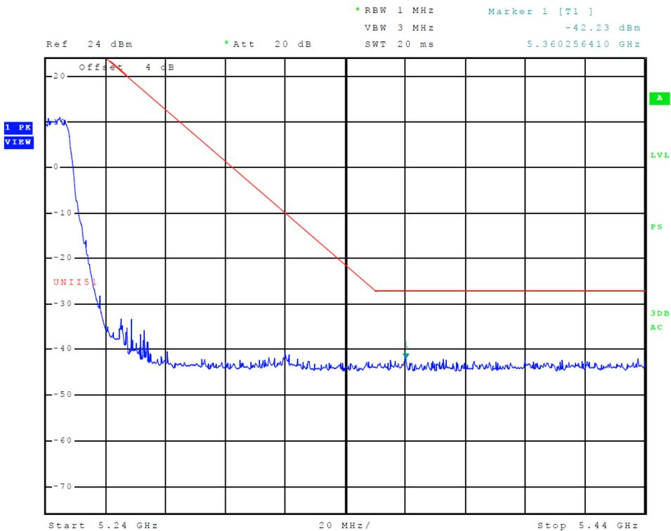
Figure 12 Plot of Transmitter High Band Edge (5150-5250 MHz Band, Chain 1, 802.11a)
