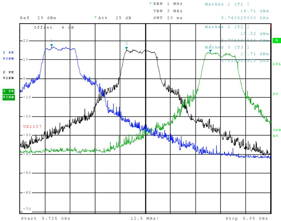
Figure 23 Plot of Transmitter Emissions (Across 5725-5850 MHz Band, Chain 0, 802.11a)
