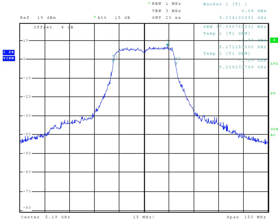
**Figure 20 Plot of Transmitter Emissions (5150-5250 MHz Band, 802.11n40, Chain 1, 99% OBW)**
