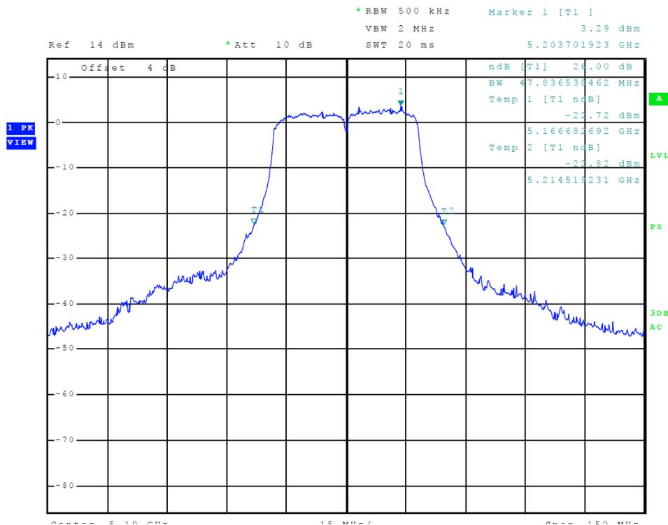
Figure 22 Plot of Transmitter Emissions (5150-5250 MHz Band, 802.11n40, Chain 1, 26 dB OBW)
