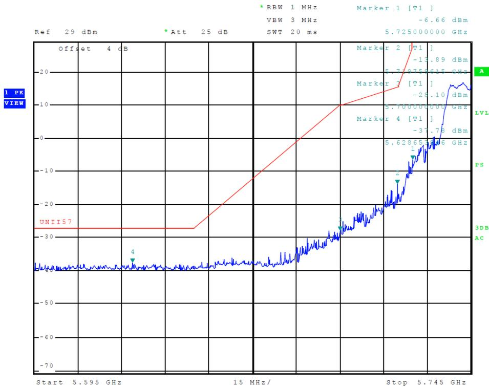
**Figure 27 Plot of Transmitter Low Band Edge (5725-5850 MHz Band, Chain 0, 802.11a)**
