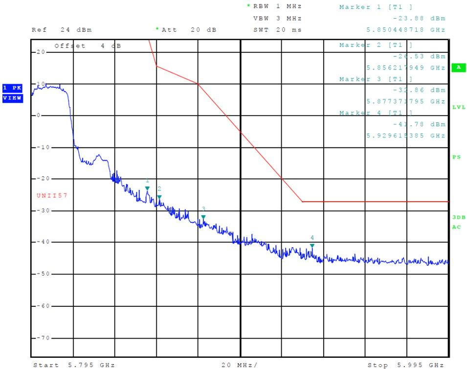
**Figure 34 Plot of Transmitter High Band Edge (5725-5850 MHz Band, Chain 1, 802.11n40)**
