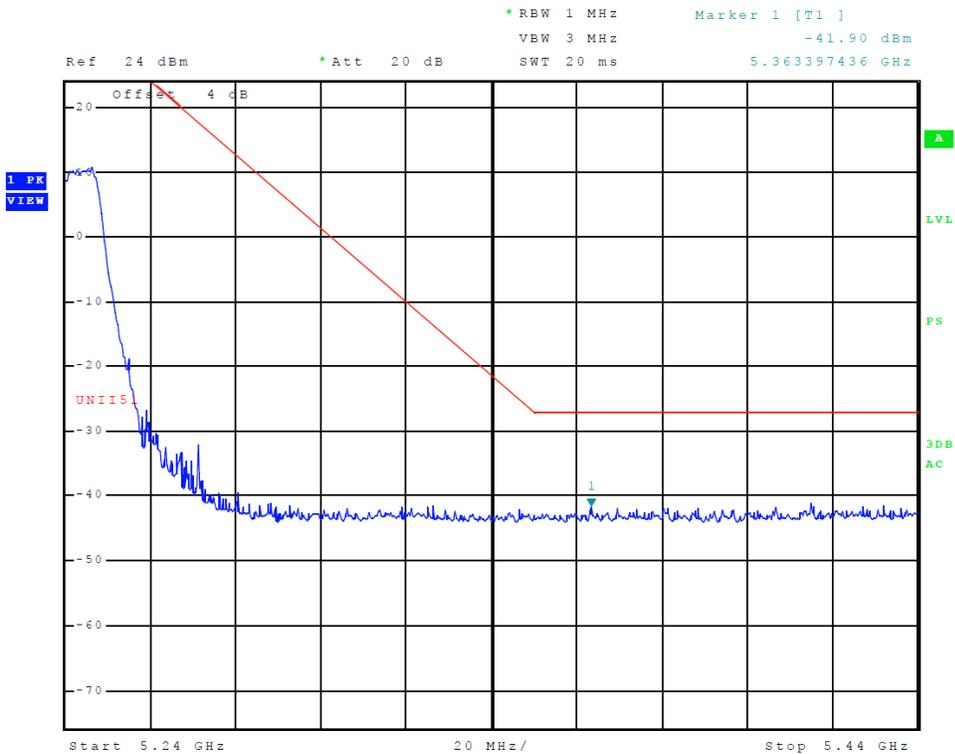
Figure 11 Plot of Transmitter High Band Edge (5150-5250 MHz Band, Chain 0, 802.11a)
