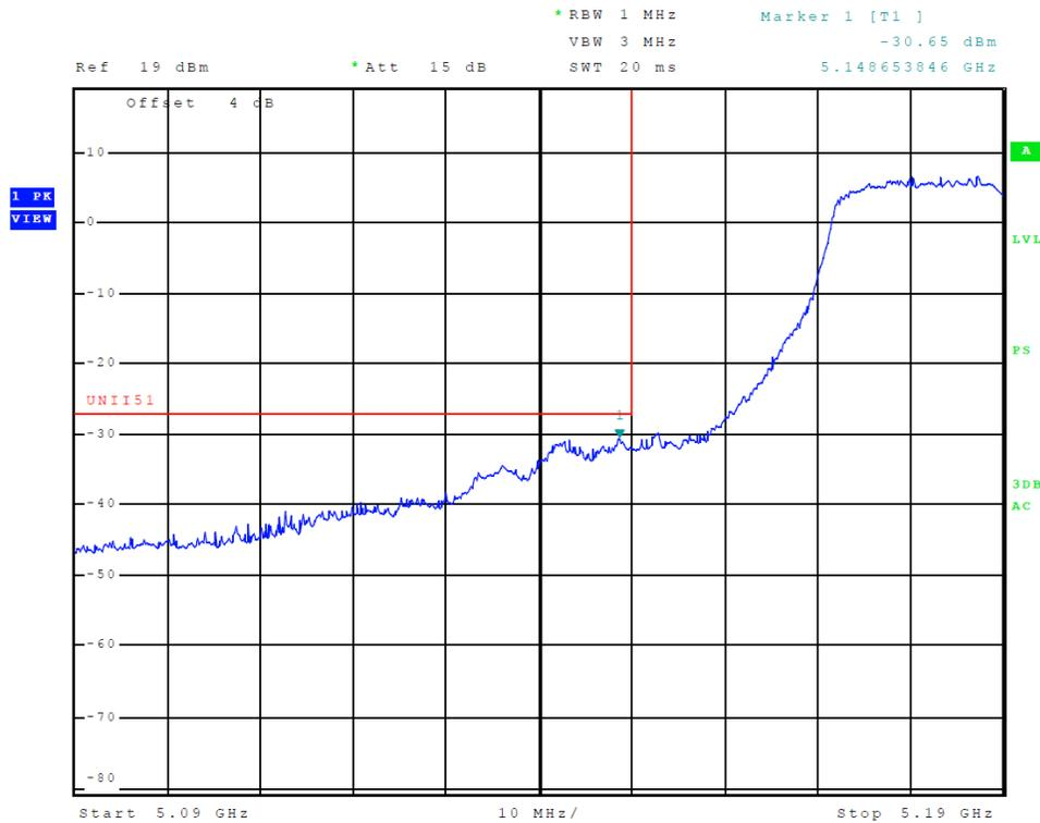
**Figure 10 Plot of Transmitter Low Band Edge (5150-5250 MHz Band, Chain 1, 802.11n40)**
