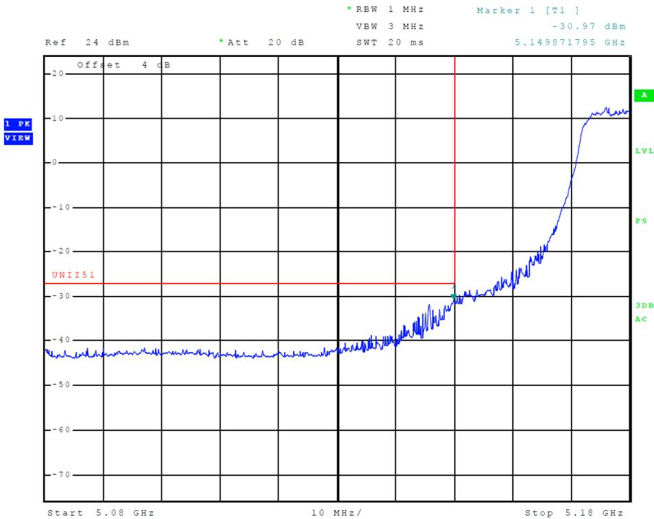
**Figure 8 Plot of Transmitter Low Band Edge (5150-5250 MHz Band, Chain 1, 802.11a)**
