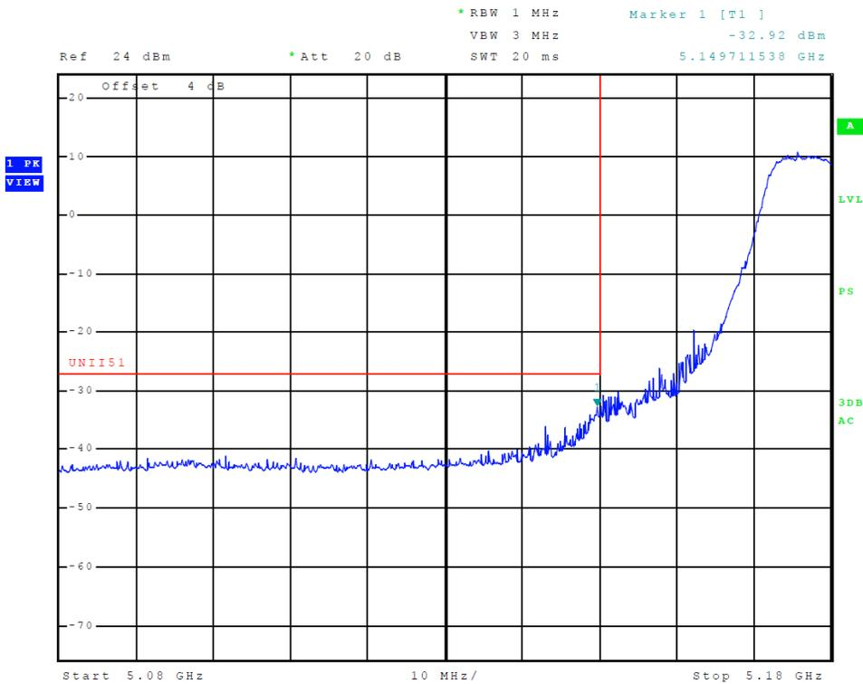
**Figure 7 Plot of Transmitter Low Band Edge (5150-5250 MHz Band, Chain 0, 802.11a)**
