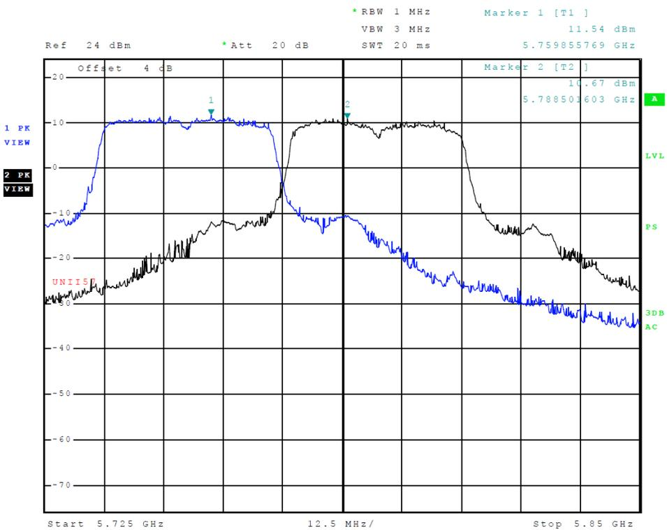
**Figure 26 Plot of Transmitter Emissions (Across 5725-5850 MHz Band, Chain 1, 802.11n40)**
