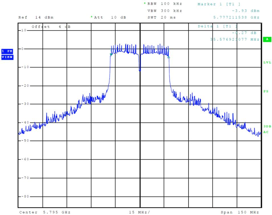
**Figure 42 Plot of Transmitter Emissions (5725-5850 MHz Band, 802.11n40, Chain 1, 6-dB OBW)**
