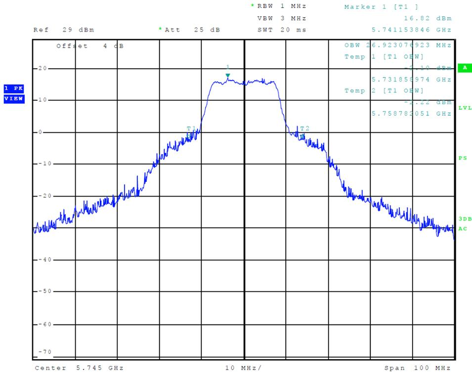
Figure 35 Plot of Transmitter Emissions (5725-5850 MHz Band, 802.11a, Chain 0, 99% OBW)
