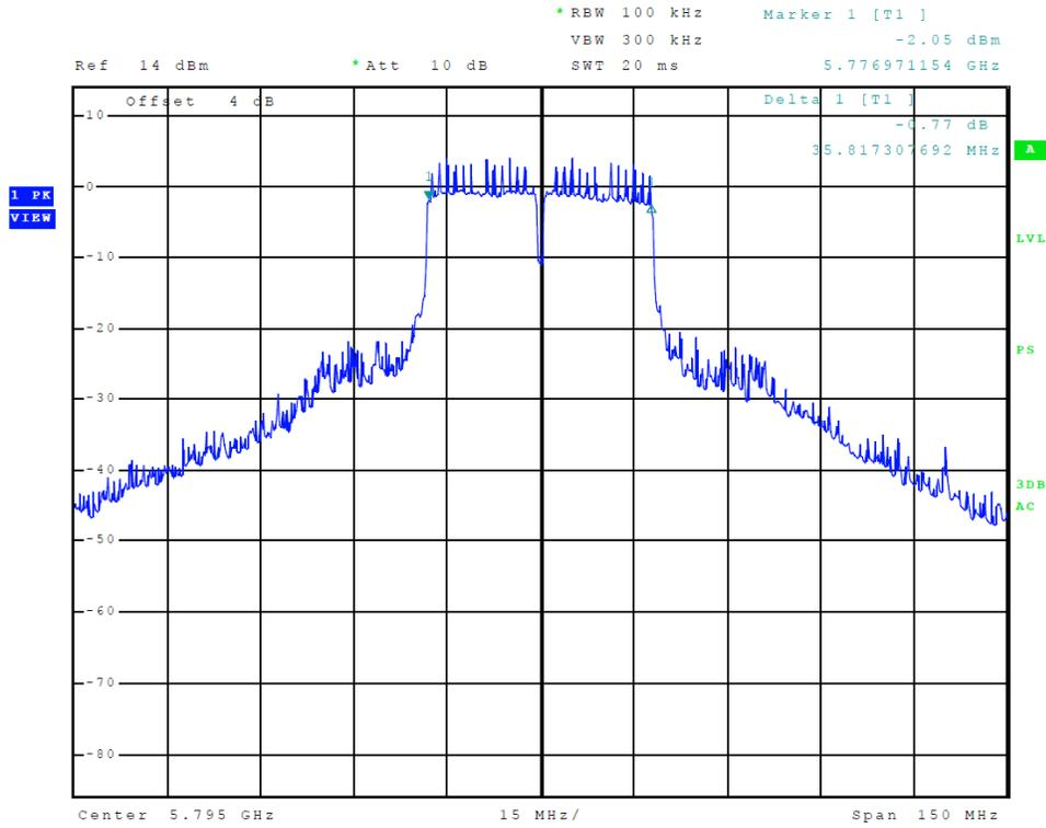
**Figure 41 Plot of Transmitter Emissions (5725-5850 MHz Band, 802.11n40, Chain 0, 6-dB OBW)**
