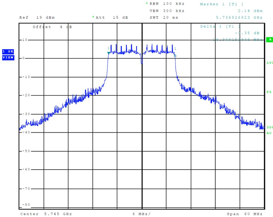
**Figure 37 Plot of Transmitter Emissions (5725-5850 MHz Band, 802.11a, Chain 0, 6-dB OBW)**
