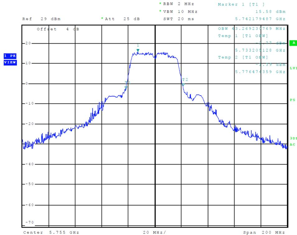
**Figure 40 Plot of Transmitter Emissions (5725-5850 MHz Band, 802.11n40, Chain 1, 99% OBW)**
