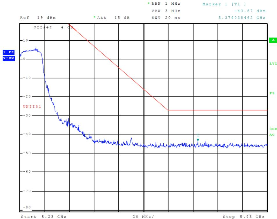
**Figure 14 Plot of Transmitter High Band Edge (5150-5250 MHz Band, Chain 1, 802.11n40)**
