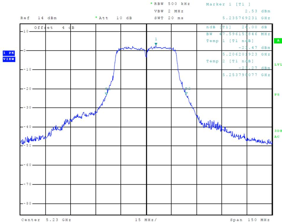
Figure 21 Plot of Transmitter Emissions (5150-5250 MHz Band, 802.11n40, Chain 0, 26 dB OBW)
