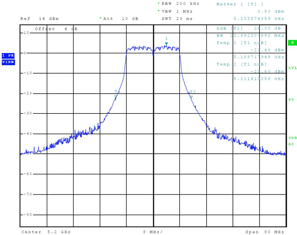
Figure 17 Plot of Transmitter Emissions (5150-5250 MHz Band, 802.11a, Chain 0, 26 dB OBW)
