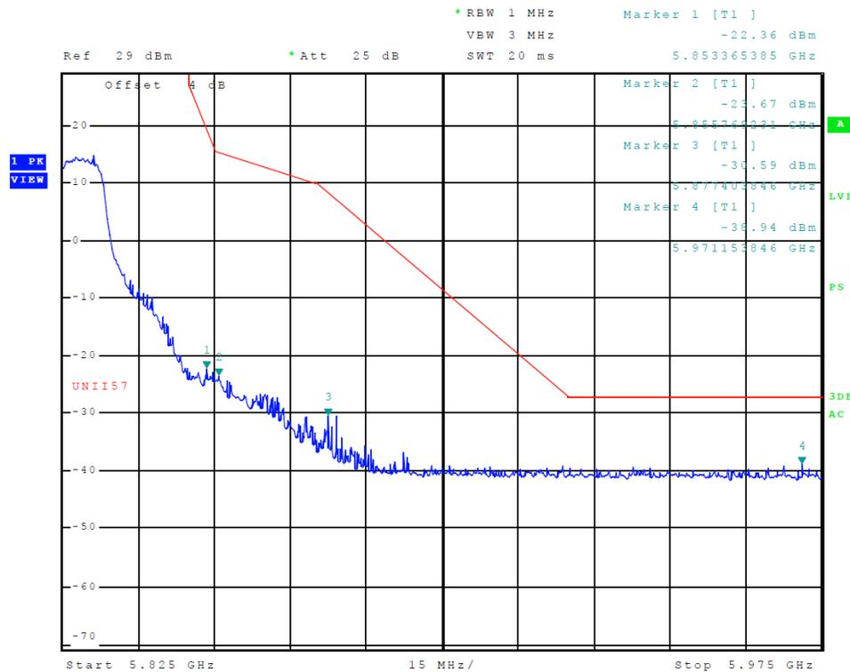
Figure 32 Plot of Transmitter High Band Edge (5725-5850 MHz Band, Chain 1, 802.11a)
