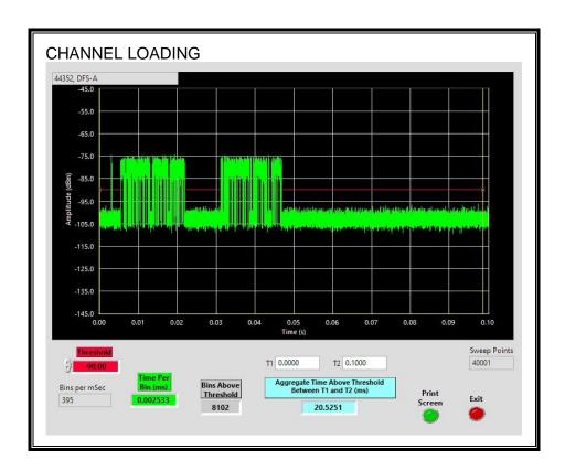
The level of traffic loading on the channel by the EUT is 20.5251%
