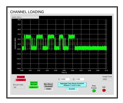
The level of traffic loading on the channel by the EUT is 34.4103%
