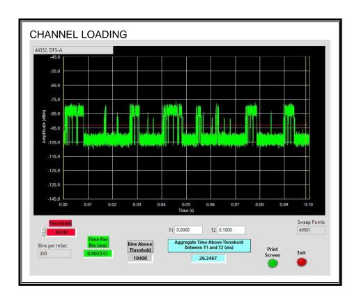
The level of traffic loading on the channel by the EUT is 26.3467%
