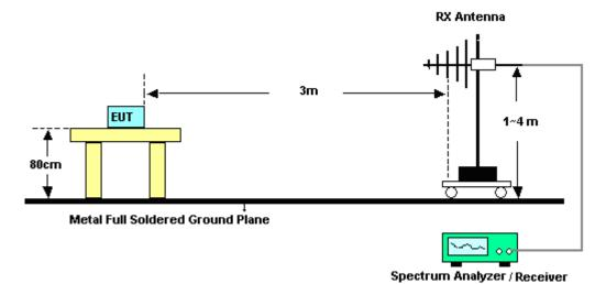
For radiated test above 1GHz
