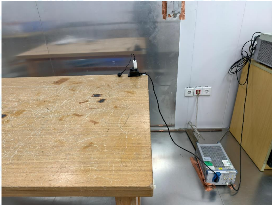
Photo of Setup for Conducted Emission (Charging Box2#)
