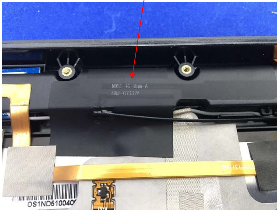
LTE/WCDMA Main Antenna
