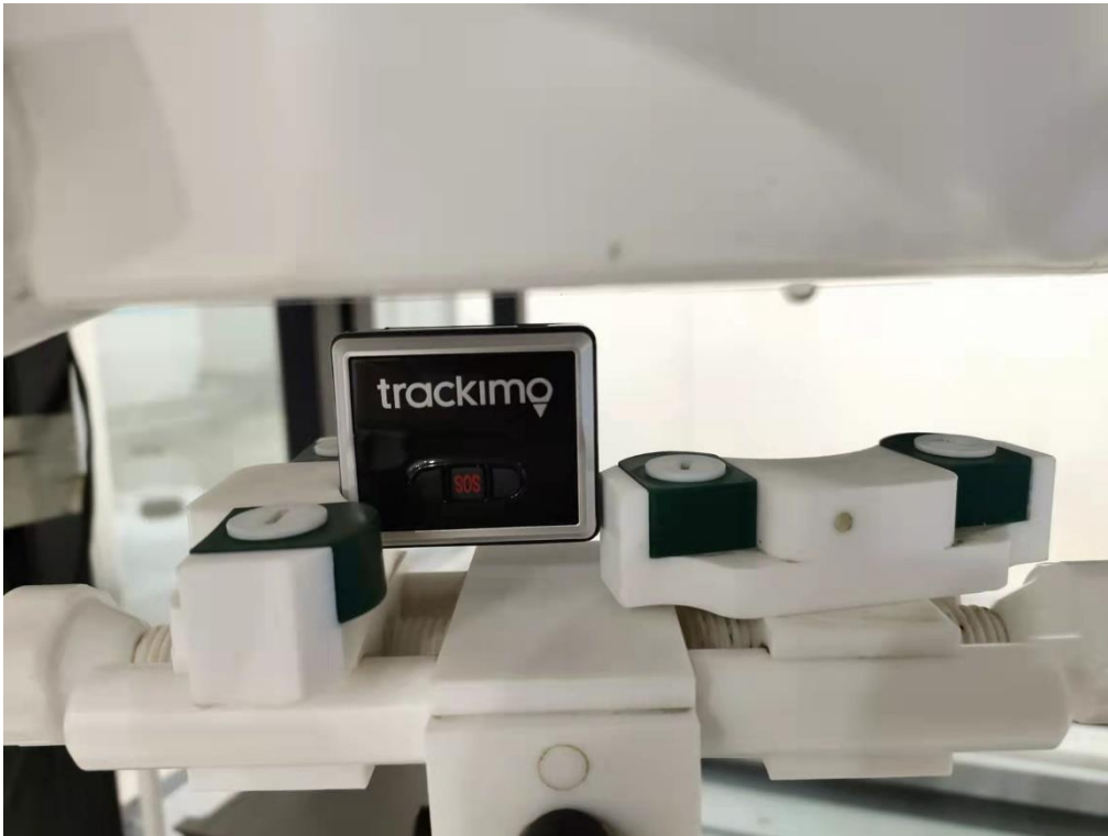
Body Top side(separation distance is 5mm)
