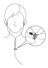
• Attach the clip to the headset cable below the remote. Position the clip so that you can speak into the microphone for taking calls hands-free, once the headset is fastened to your clothes.
