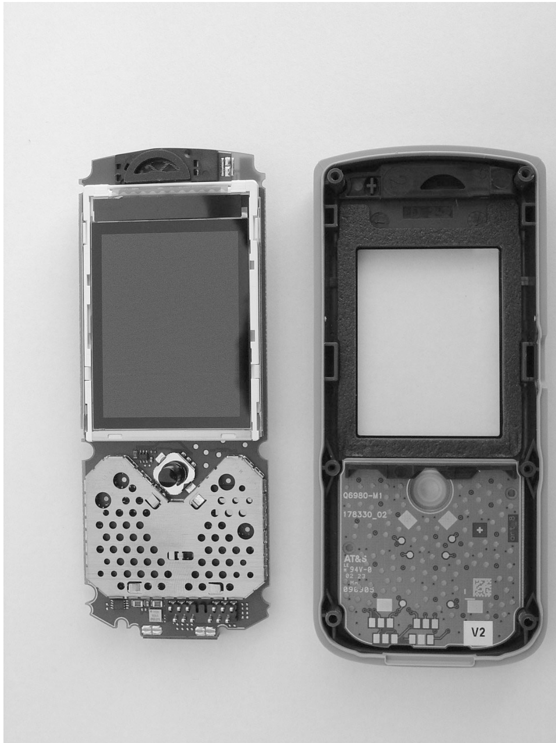
ME75 Disassembly Step 2
