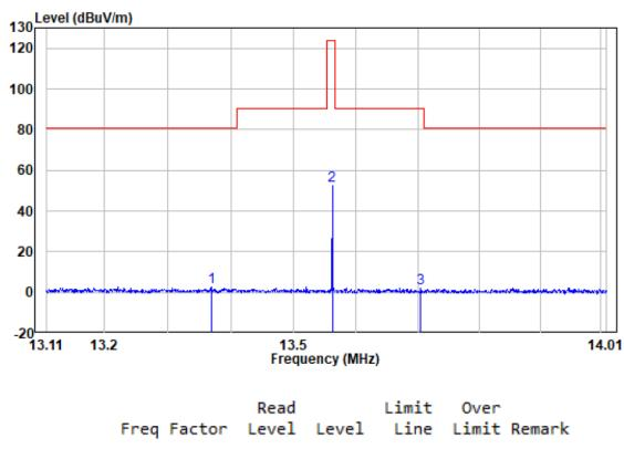
2) Emission Mask & Fundamental: (worst case is coaxial polarization)
