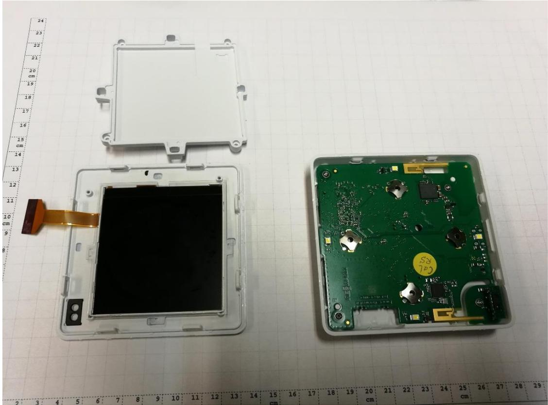
Photograph 4: ViCare Thermostat – Housing Top Side – Display Front
