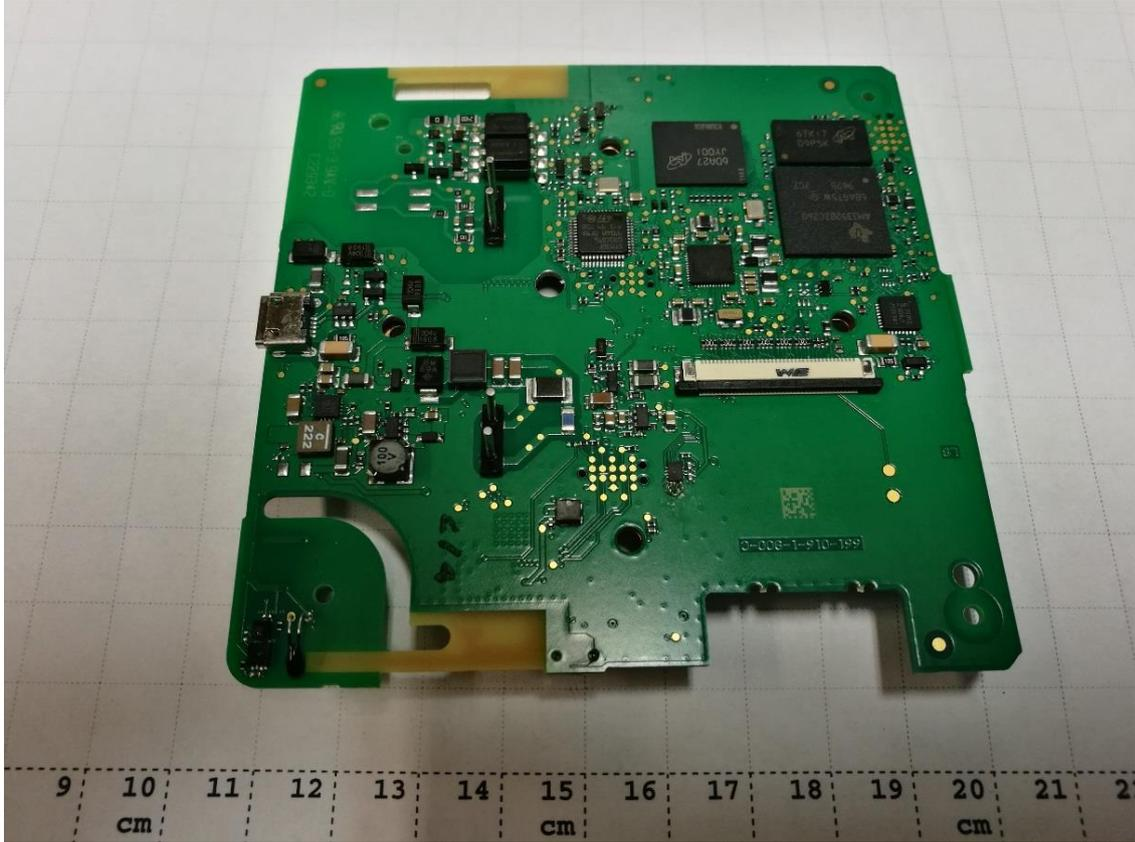
Photograph 6: ViCare Thermostat – Main PCB Bottom Side
