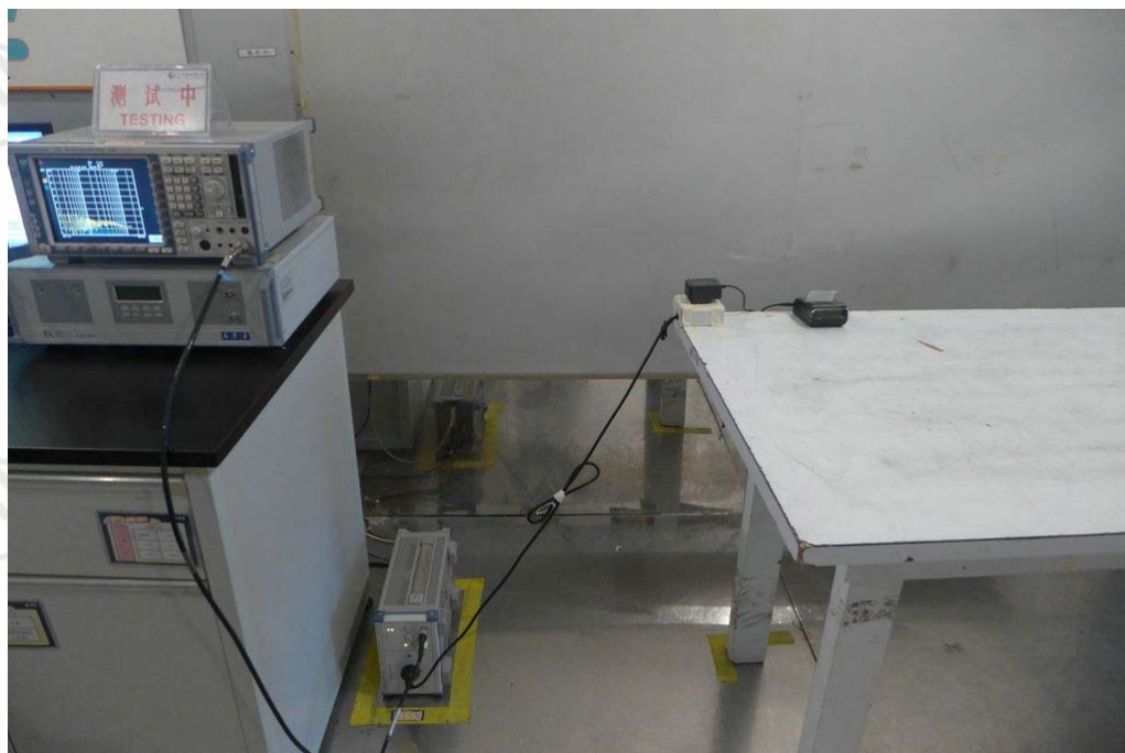
Conducted Emissions Test Setup
