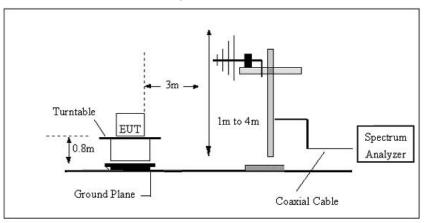
(C) Radiated Emission Test-Up Frequency Above 1GHz
