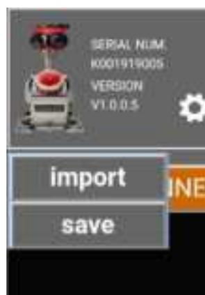
Click **save** will save opened real-time trajectory as a kml file. In below prompt box, input a file name and click **OK** to save trajectory for next time use.
