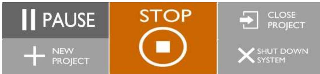
During data capture process, if vehicle faces red light or traffic jam need to stop, the **PAUSE** button can be chosen to click which can stop data recording (scanner still work); When it can be captured normally, click **CONTINUE** to keep capture.
