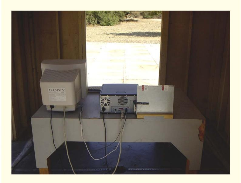
Radiated Emissions Measurement (Rear View) Setup
