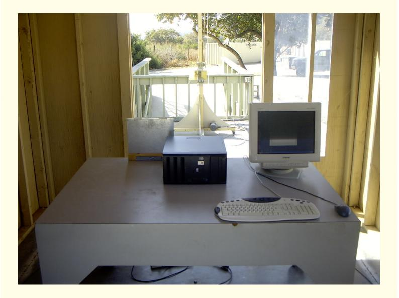
Radiated Emissions Measurement (Front View) Setup
