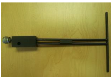
Figure 1 – MVG COMOSAR Validation Dipole
