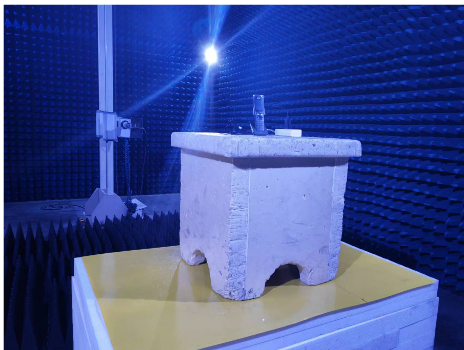
Photo of Radiated Emission Measurement (Above 1G)
