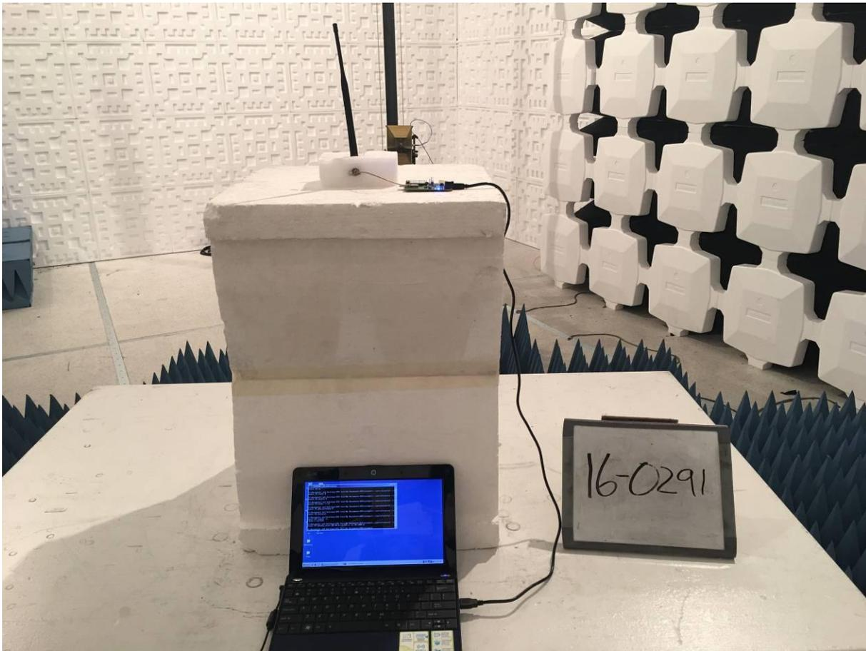
**Figure 1. Intentional Radiated Emissions, Close-Up and Above 1GHz Test Setup**
