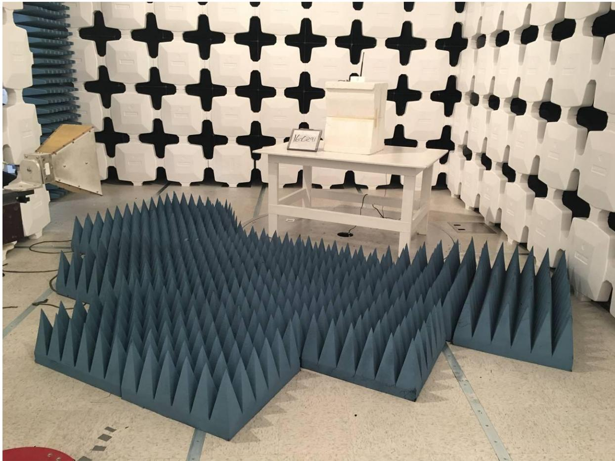
**Figure 2. Intentional Radiated Emissions Fundamental and Harmonics Testing**
