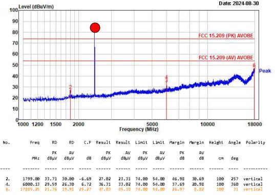
Remarks: C.F (Correction Factor) = Antenna factor + Cable loss - Preamp gain
