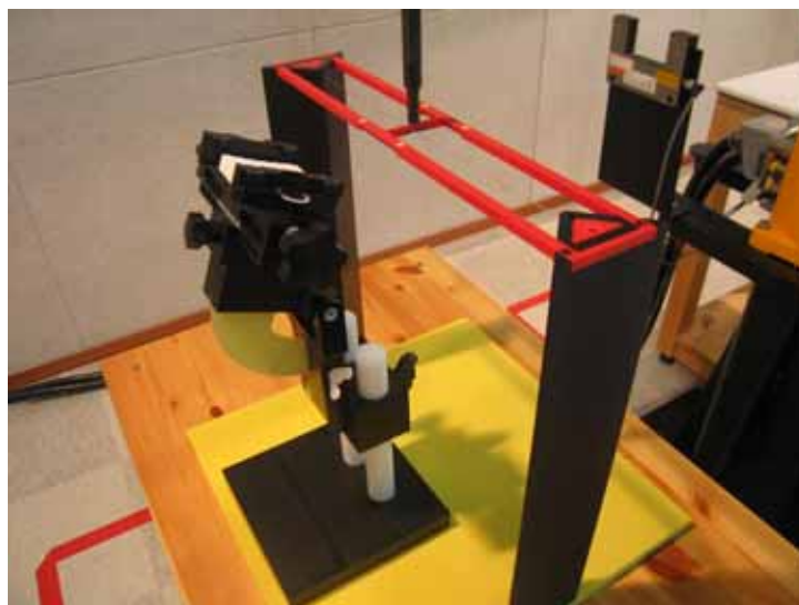
Figure 2. HAC Phantom & Device Holder
