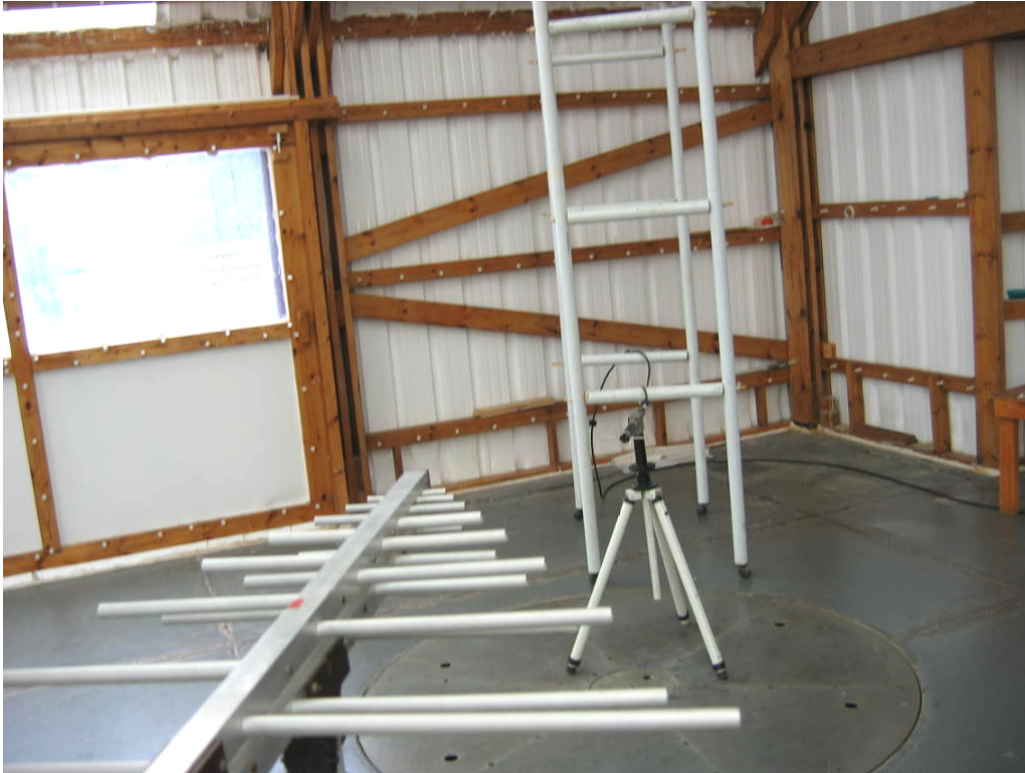
Photograph No.2 Substitution method measurement setup
