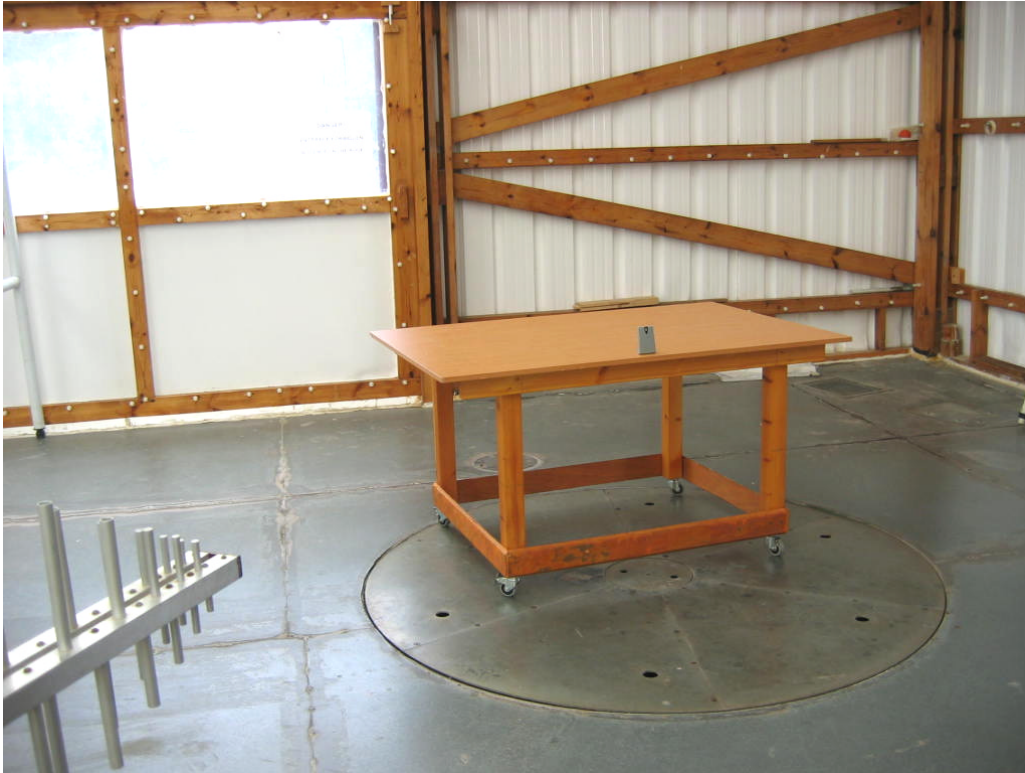
Photograph No.1 Output power and occupied bandwidth measurement setup
