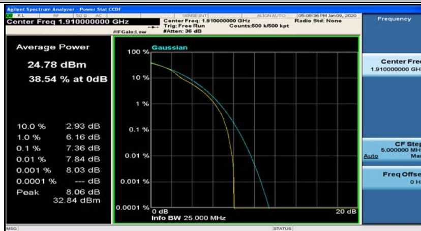
Channel Bandwidth: 10 MHz_HCH_16QAM_1RB#24
