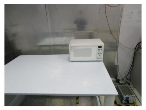
1.2 Radiated Emissions (30MHz-1GHz) Test Setup
