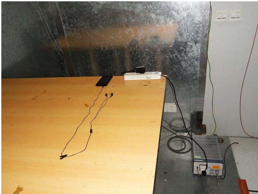
Conducted Emission Test Setup:
