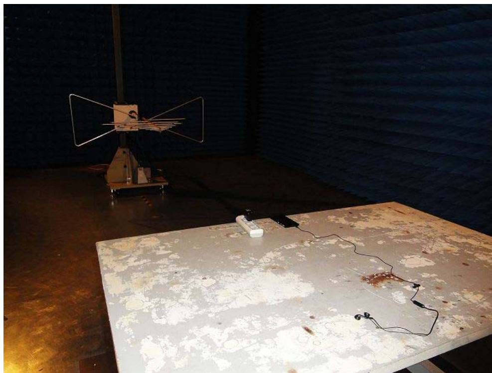
Radiated Emission Test Setup:
