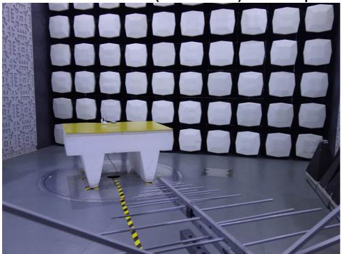
1.3 Radiated Emissions (below 30MHz) Test Setup
