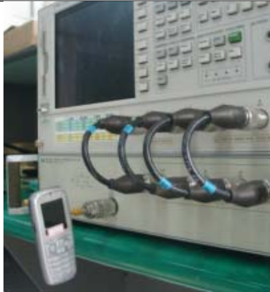
Figure 1: Testing with network analyzer
