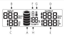
A: Battery Level B: Remaining Charging Time C: Input Power
