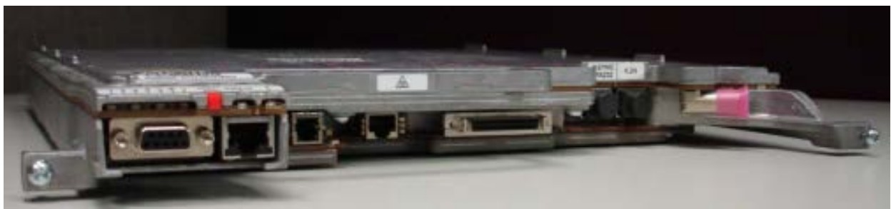
Transceiver Module with the Transceiver Option Card (TOC) Installed
