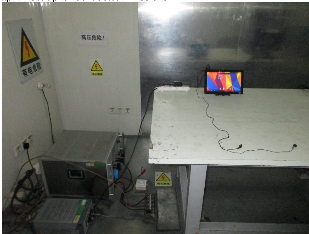
Photograph 2: Set-up for Spurious Emissions for below 30MHz
