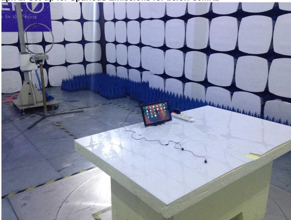
Photograph 2: Set-up for Spurious Emissions for below 30MHz
