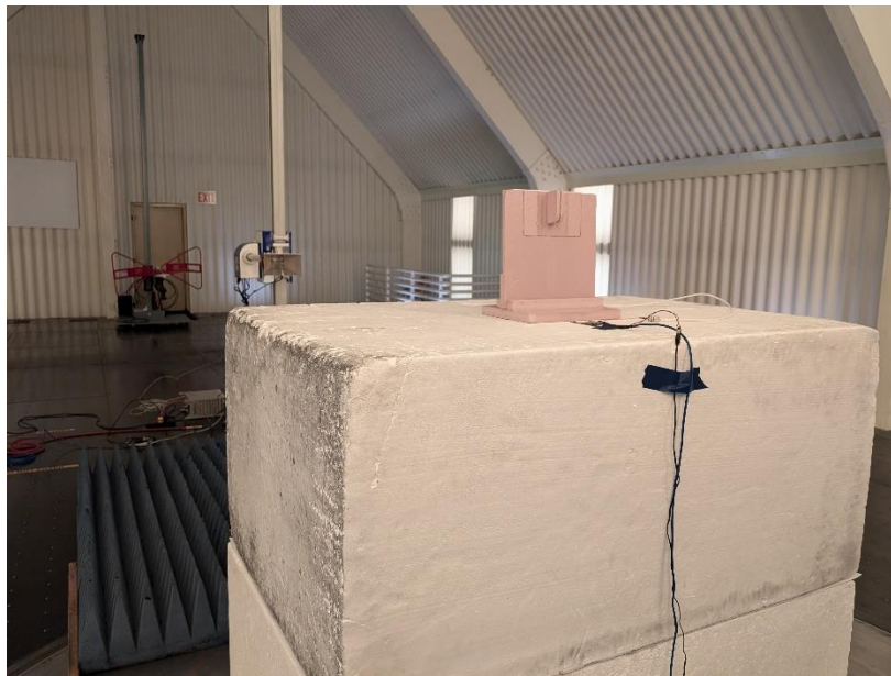
Photograph 12: Back View Radiated Emissions Worst-Case Configuration 900 MHz Patch Antenna – Frequencies Above 1000 MHz
