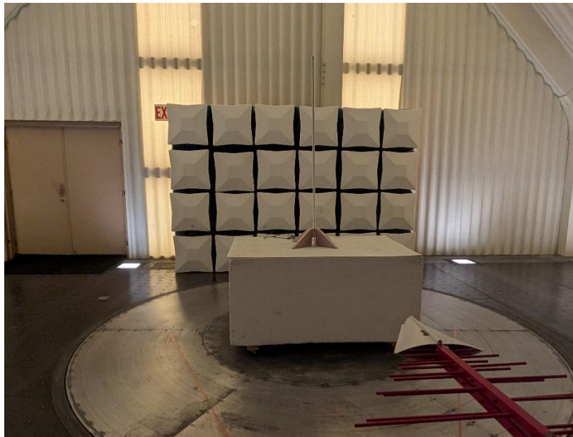
Photograph 5: Front View Radiated Emissions Worst-Case Configuration 900 MHz Monopole Antenna – Frequencies Below 1000 MHz
