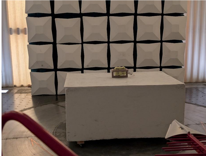
Photograph 1: Front View Radiated Emissions Worst-Case Configuration 900 MHz Internal Antenna – Frequencies Below 1000 MHz
