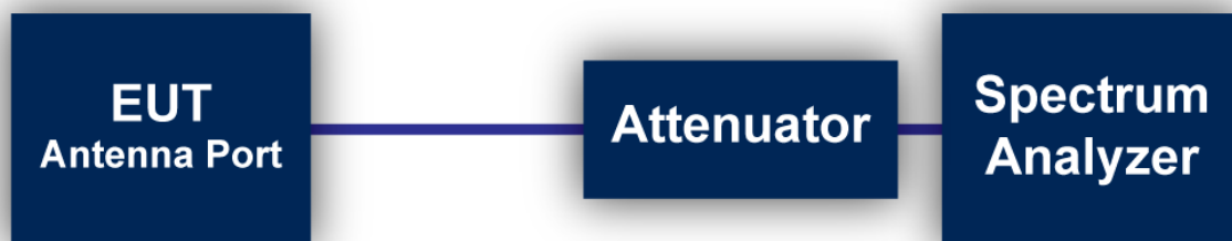
Figure 2: Direct Connection at the Antenna Port Test
