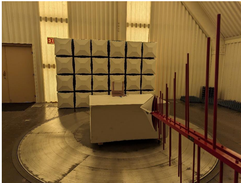
Photograph 9: Front View Radiated Emissions Worst-Case Configuration 900 MHz Patch Antenna – Frequencies Below 1000 MHz
