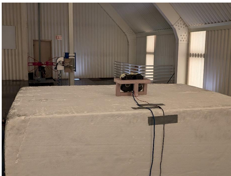
Photograph 4: Back View Radiated Emissions Worst-Case Configuration 900 MHz Internal Antenna – Frequencies Above 1000 MHz
