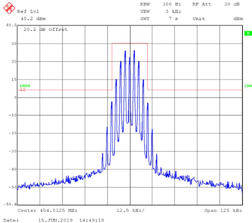
**4FSK,12.5kHz,High Power - Frequency 454.0125 MHz: 99% Occupied & 26 dB Bandwidth**
