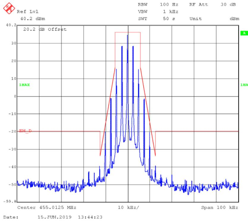
**FM,12.5kHz,Low Power - Frequency 455.0125 MHz: 99% Occupied & 26 dB Bandwidth**
