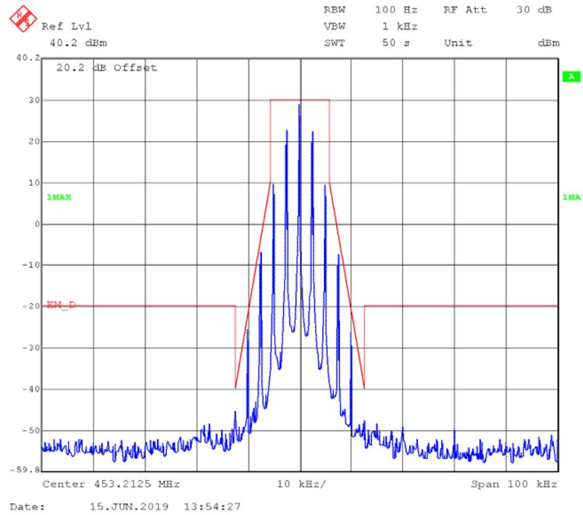
**4FSK,12.5kHz,High Power - Frequency 453.2125 MHz: 99% Occupied & 26 dB Bandwidth**
