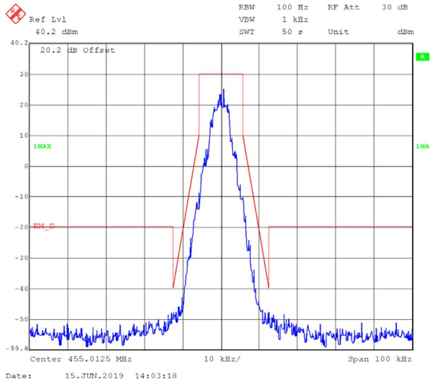
**Part 22****FM,12.5kHz,High Power - Frequency 454.0125 MHz: 99% Occupied & 26 dB Bandwidth**
