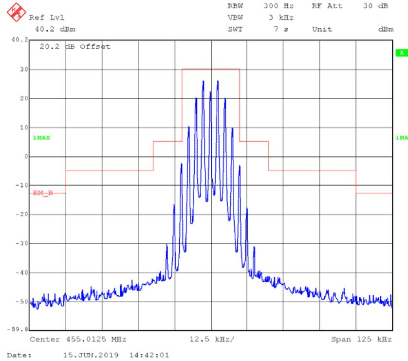
**4FSK,12.5kHz,High Power - Frequency 455.0125 MHz: 99% Occupied & 26 dB Bandwidth**
