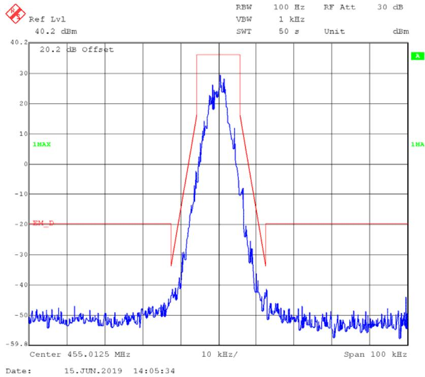
**4FSK,12.5kHz,Low Power - Frequency 450.03125 MHz: 99% Occupied & 26 dB Bandwidth**
