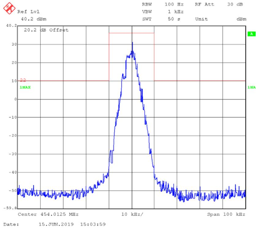
**4FSK,12.5kHz,Low Power - Frequency 454.0125 MHz: 99% Occupied & 26 dB Bandwidth**
