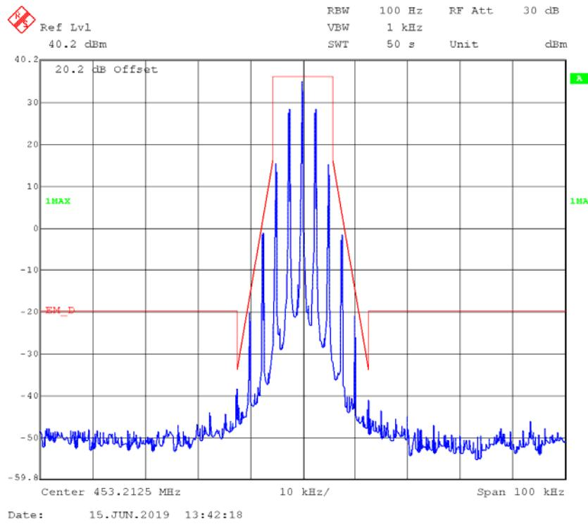
**FM,12.5kHz,Low Power - Frequency 453.2125 MHz: 99% Occupied & 26 dB Bandwidth**
