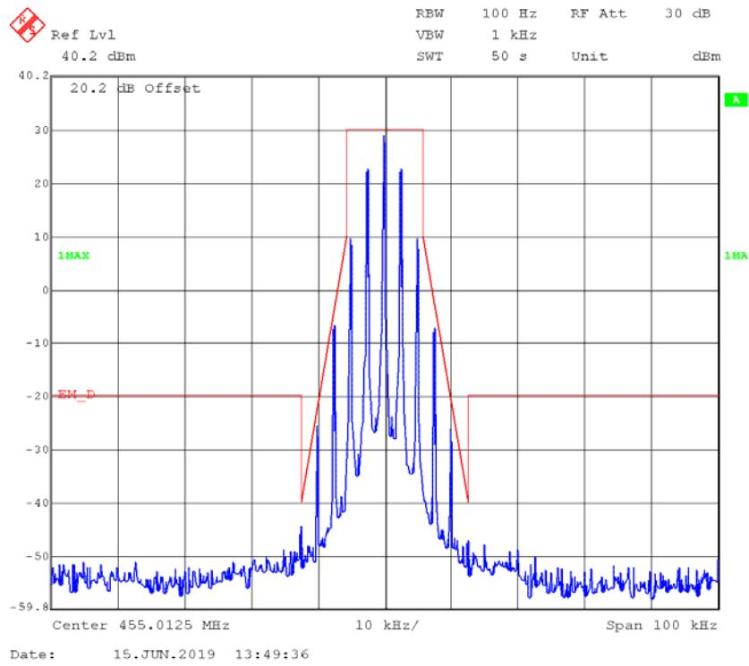
**FM,25kHz,High Power - Frequency 455.0125 MHz: 99% Occupied & 26 dB Bandwidth**
