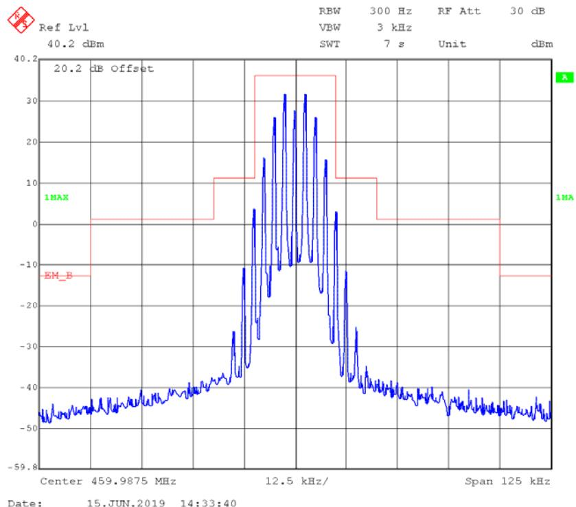
**FM,25kHz,Low Power - Frequency 459.9875 MHz MHz: 99% Occupied & 26 dB Bandwidth**
