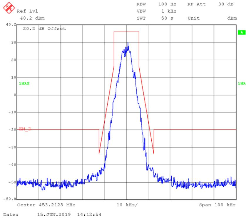
**4FSK,12.5kHz,Low Power - Frequency 453.2125 MHz: 99% Occupied & 26 dB Bandwidth**
