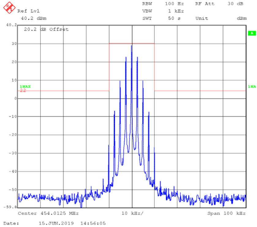
**FM,25kHz,High Power - Frequency 454.0125 MHz: 99% Occupied & 26 dB Bandwidth**
