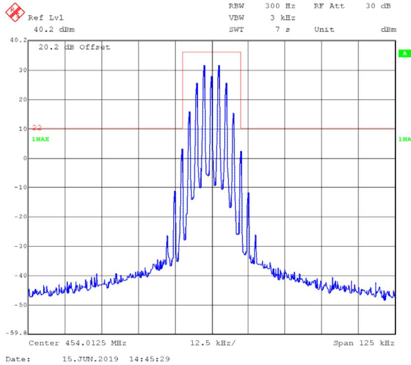
**FM,25kHz,Low Power - Frequency 454.0125 MHz: 99% Occupied & 26 dB Bandwidth**
