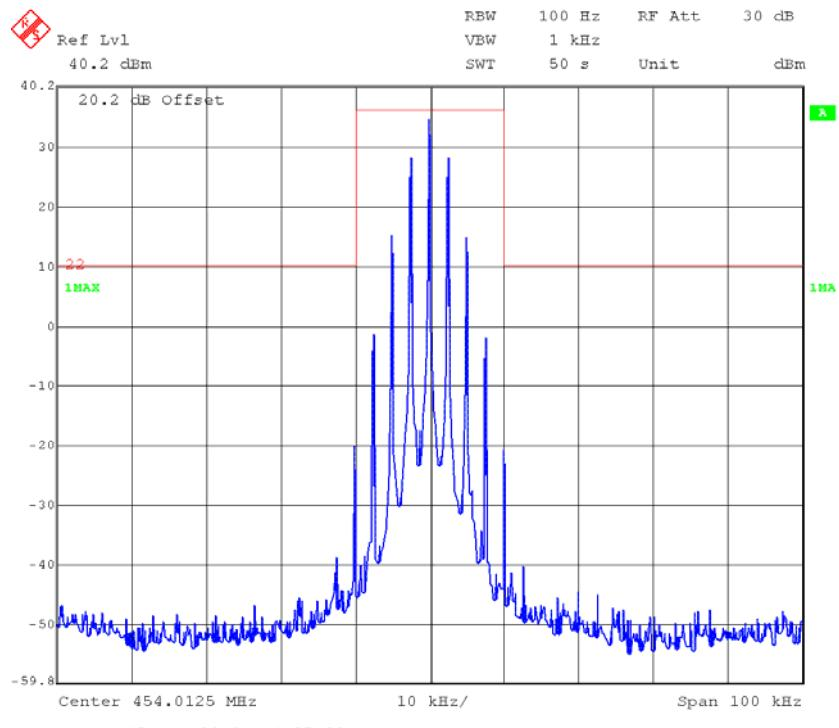
**FM,12.5kHz,Low Power - Frequency 454.0125 MHz: 99% Occupied & 26 dB Bandwidth**
