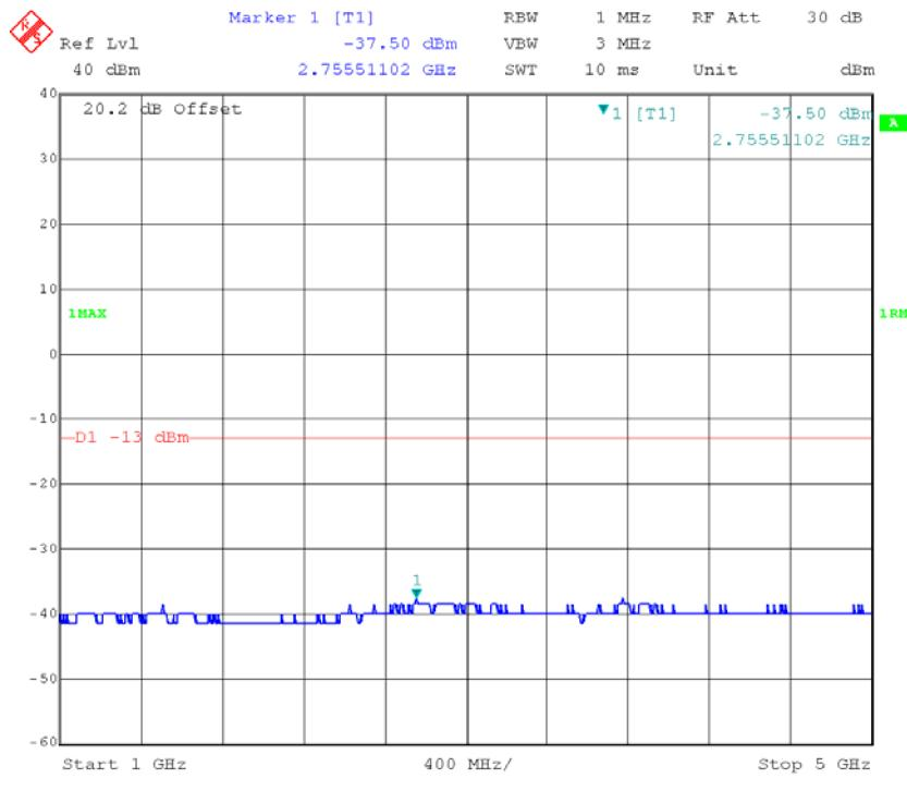
**25kHz,FM, High power:****30MHz – 1 GHz, Channel Spacing 25 kHz, 454.0125 MHz**
