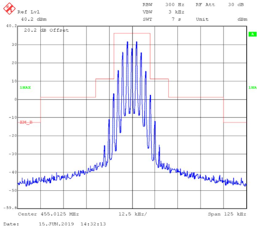
**FM,25kHz,Low Power - Frequency 455.0125 MHz: 99% Occupied & 26 dB Bandwidth**
