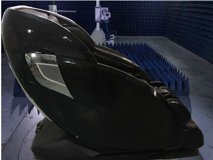
Photograph of set-up for Radiated Emission above 18-25GHz
