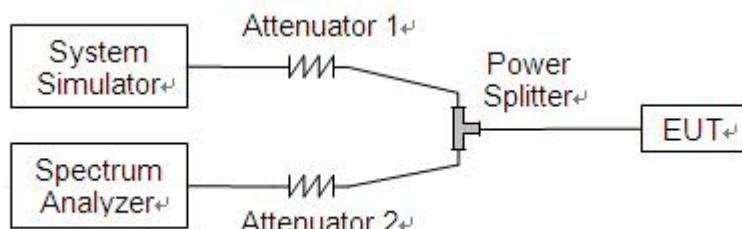
The EUT is coupled to the Spectrum Analyzer (SA) and the System Simulator (SS) with Attenuators through the Power Splitter; the RF load attached to the EUT antenna terminal is 50Ohm; the path loss as the factor is calibrated to correct the reading. The EUT is commanded by the SS to operate at the maximum output power i.e. Power Control Level (PCL) = 5 and Power Class = 4. A call is established between the EUT and the SS.
