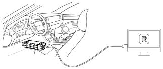
2 Ensure that the communication is normal after the connection is completed. Then open the OEM diagnostic software and select RLink as the diagnostic interface.
