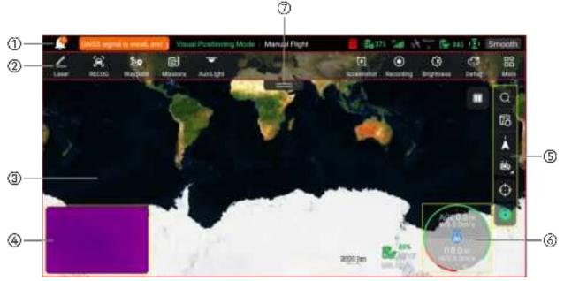
Fig 6-1 Main Interface of the Autel Enterprise Application (EVO Lite 640T Enterprise Aircraft)
