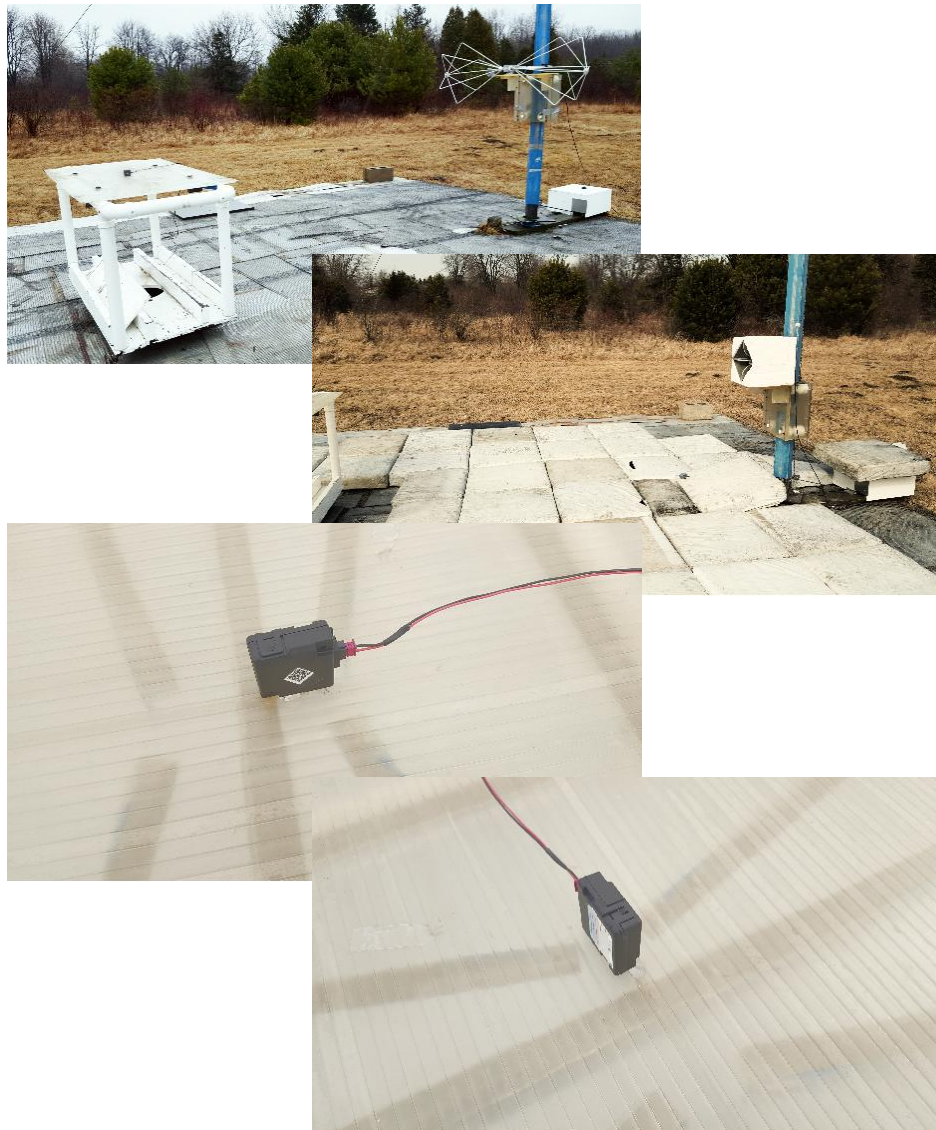
Figure 4: Radiated Emissions Test Setup Photograph(s).
