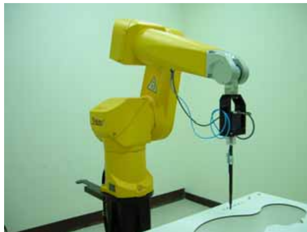
Fig. 5.2 Probe setup on robot
