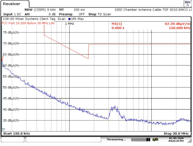
6.4.1.4 Parallel Measurement Antenna – 150 kHz to 30 MHz – 6.8 Mbps 64M
