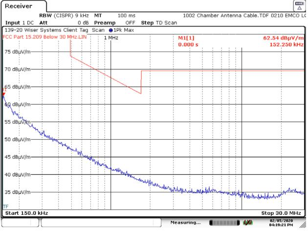
6.4.1.5 Perpendicular Measurement Antenna – 150 kHz to 30 MHz – 6.8 Mbps 64M
