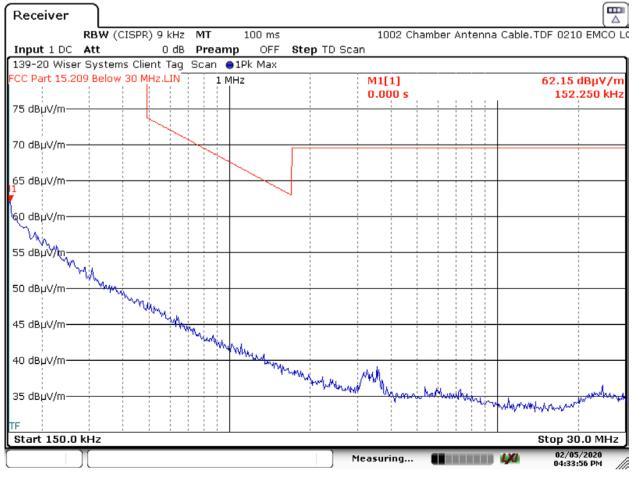
6.4.1.6 Ground Parallel Measurement Antenna – 150 kHz to 30 MHz – 6.8 Mbps 64M
