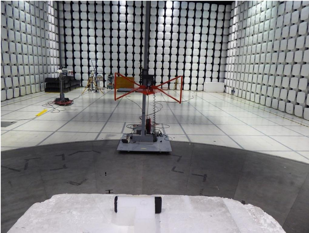
Figure 29: 30 - 1000 MHz Radiated Emission Test Setup – Front View
