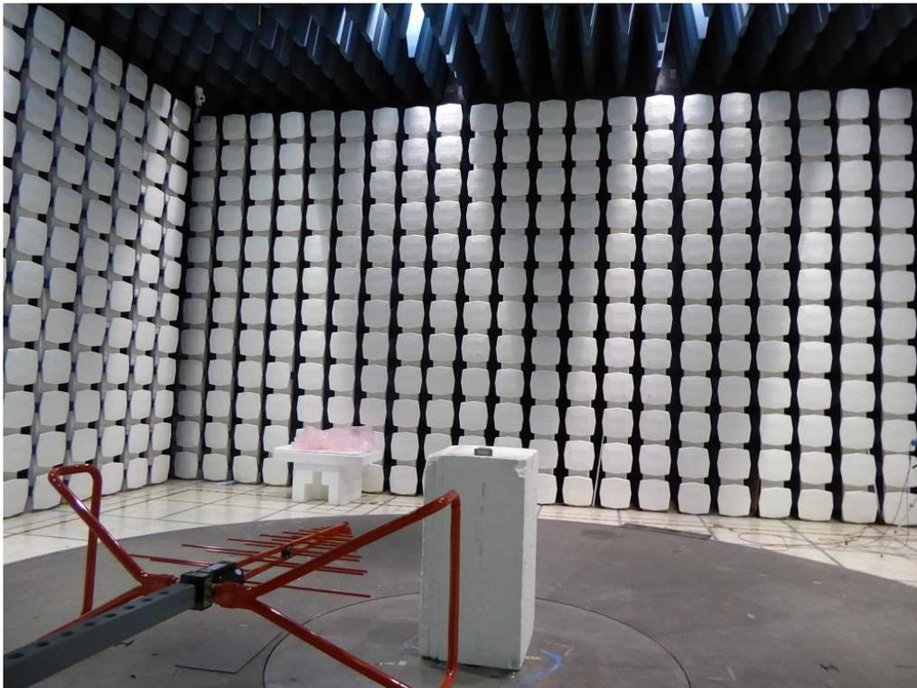
Figure 28: 30 - 1000 MHz Radiated Emission Test Setup – Rear View
