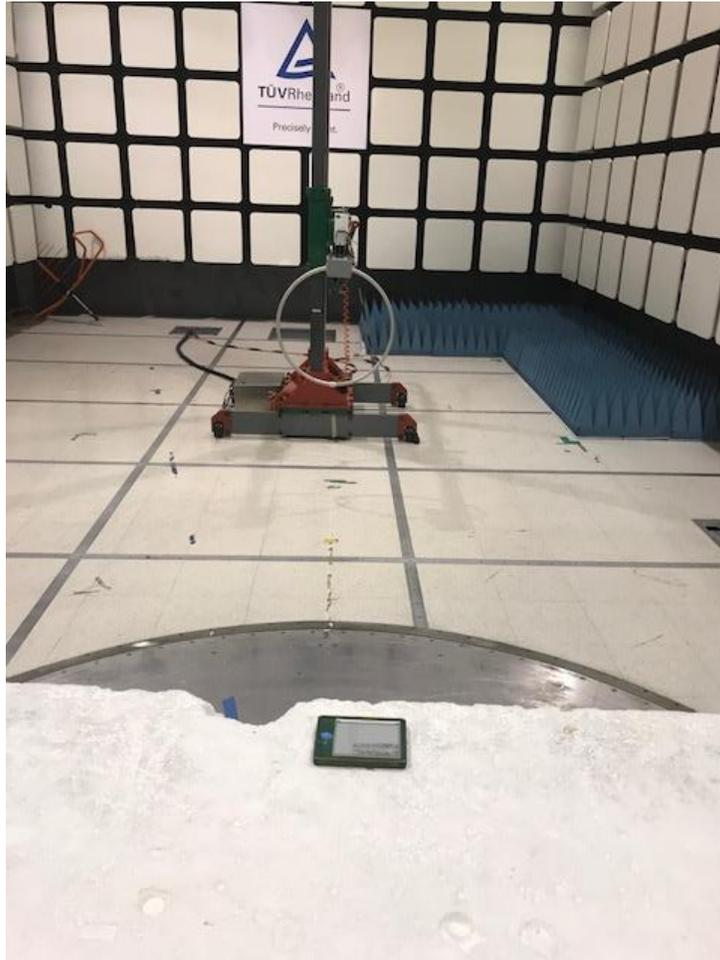
Figure 27: 9 – 30,000 kHz Radiated Emission Test Setup – Front View
