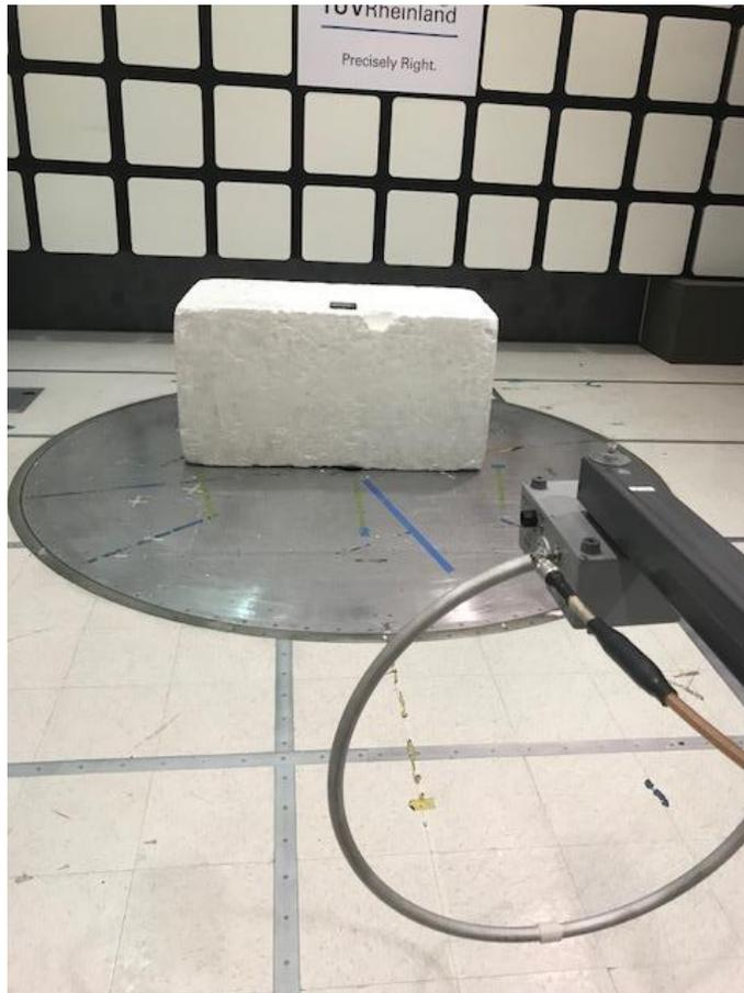
Figure 26: 9 – 30,000 kHz Radiated Emission Test Setup – Rear View
