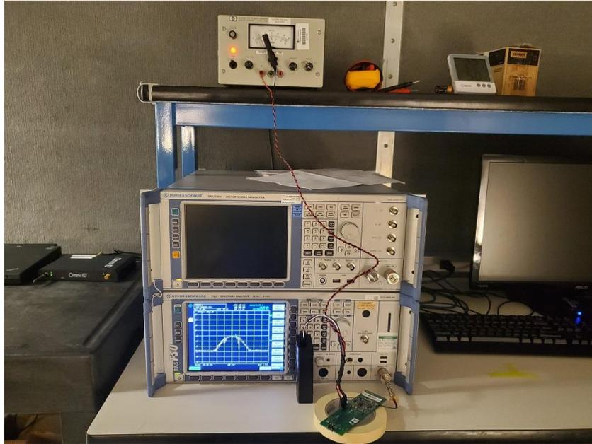
Figure 25: Photo of Conducted Tabletop Setup
